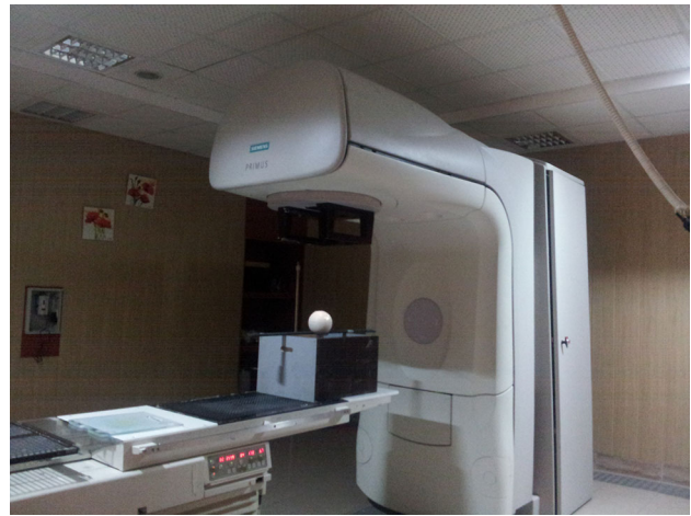
Fig. 2 Irradiation of Bonner sphere with 15 MV linac
