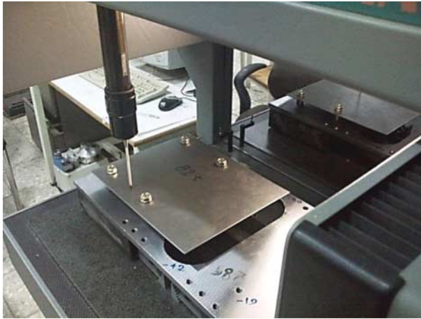
Figure 9. Surface profile digitising of a test piece.
