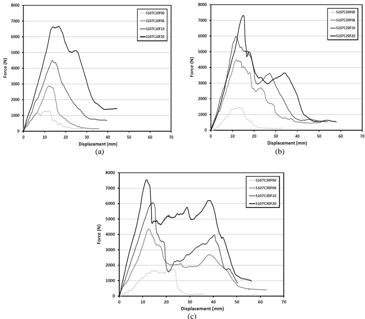
Fig. 5. Piercing force-displacement curves of specimens with  $0.7 \text{ g/cm}^3$  foam core density for a) 10 mm, b) 20 mm and c) 30 mm foam core thickness
