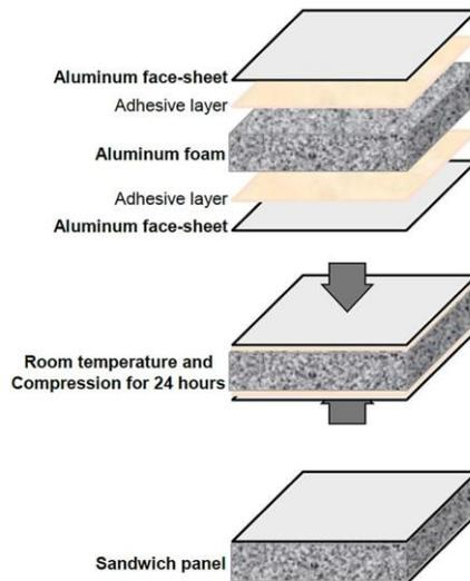
Fig. 1. Preparation procedure of the sandwich panels
