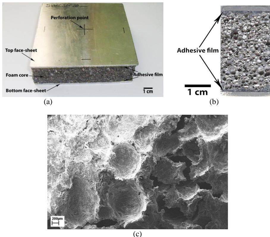
Fig. 2. a) A produced sandwich panel with its different parts, b) an image from cross section of a specimen, and c) a scanning electron micrograph of foam core fracture surface
