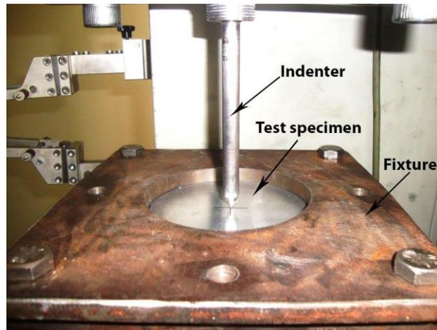
Fig. 3. Quasi-static perforation test setup
