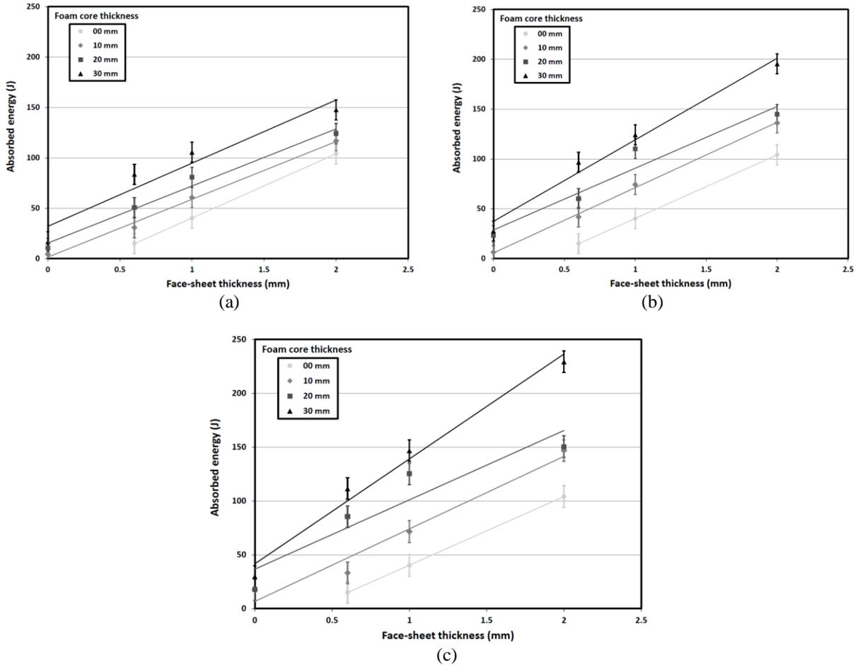
Fig. 7. Effect of face-sheet thickness on total absorbed energy of a)  $0.5 \text{ g/cm}^3$ , b)  $0.6 \text{ g/cm}^3$  and c)  $0.7 \text{ g/cm}^3$  foam core density specimens
