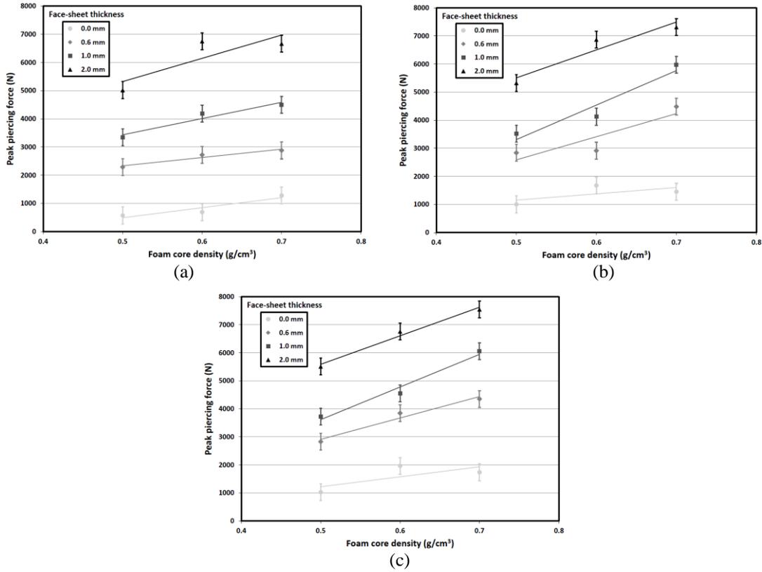
Fig. 10. Effect of foam core density on peak piercing force of specimens with a) 10 mm, b) 20 mm and c) 30 mm foam core thickness
