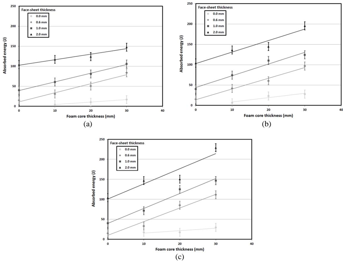
Fig. 9. Effect of foam core thickness on total absorbed energy of a) 0.5 g/cm<sup>3</sup>, b) 0.6 g/cm<sup>3</sup> and c) 0.7 g/cm<sup>3</sup> foam core density specimens
