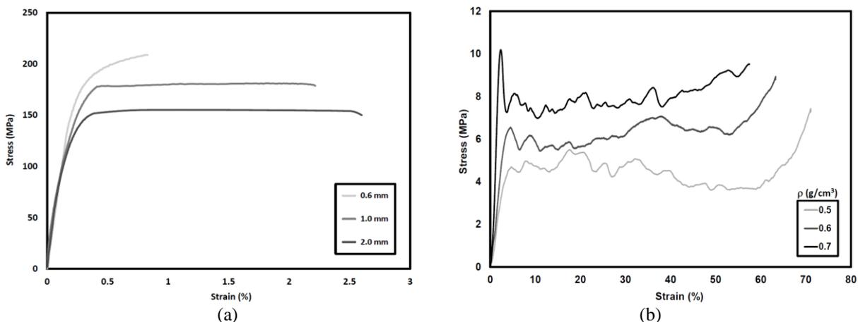
Fig. 4. Quasi-static engineering stress-strain curves of a) face-sheets and b) foam cores
