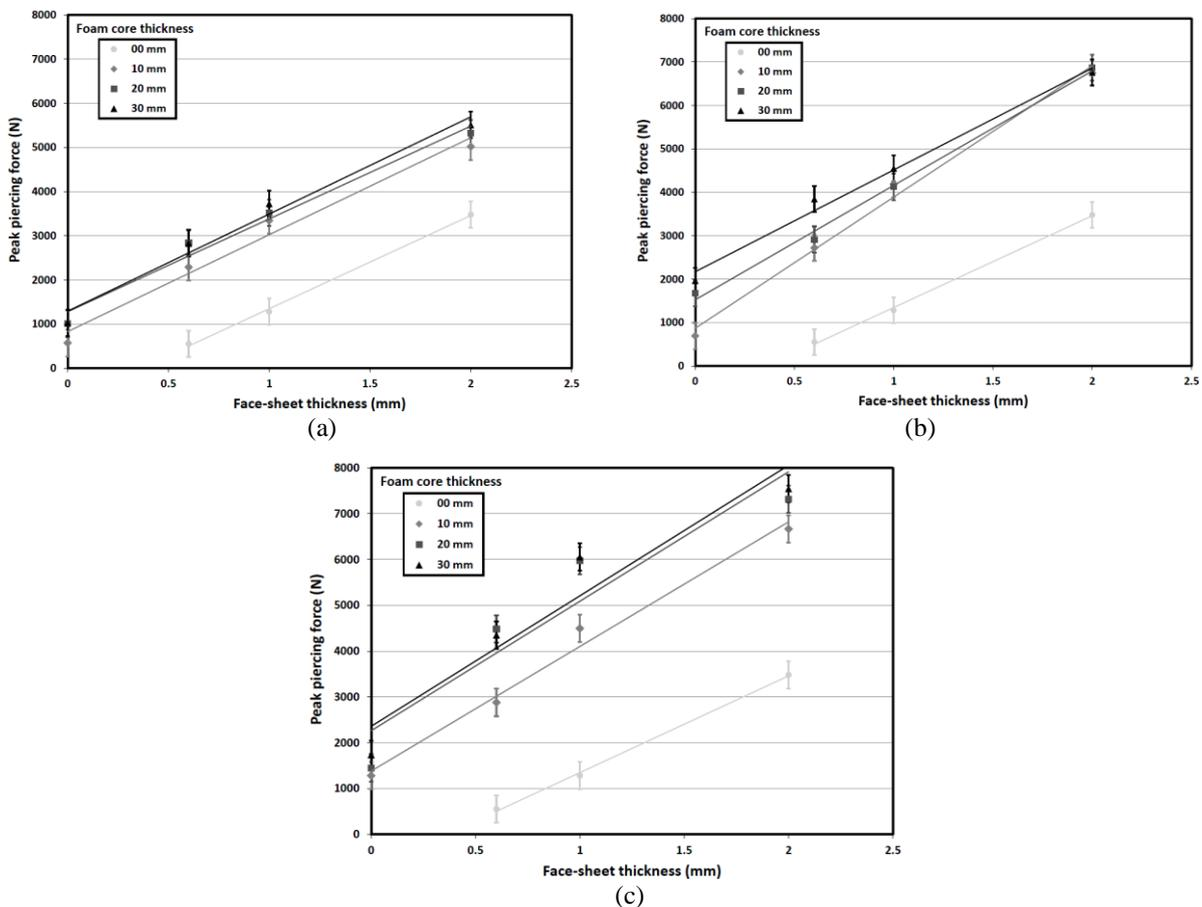
Fig. 6. Effect of face-sheet thickness on peak piercing force of a) 0.5 g/cm<sup>3</sup>, b) 0.6 g/cm<sup>3</sup> and c) 0.7 g/cm<sup>3</sup> foam core density specimens
