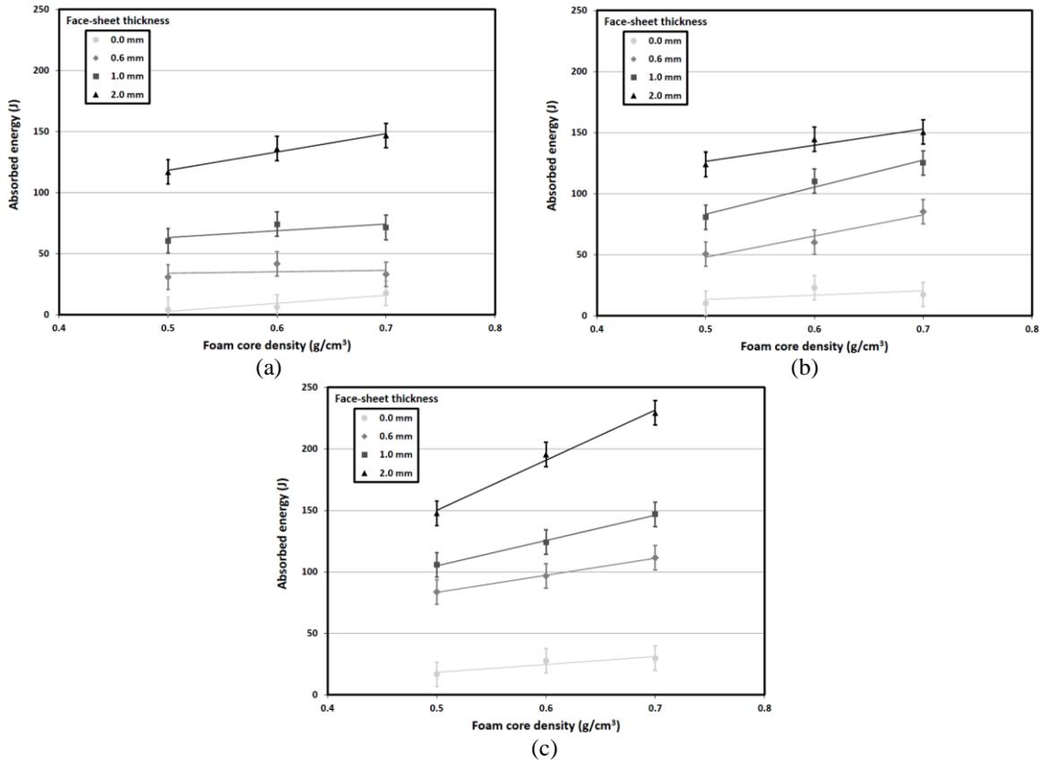
Fig. 11. Effect of foam core density on total absorbed energy of specimens with a) 10 mm, b) 20 mm and c) 30 mm foam core thickness
