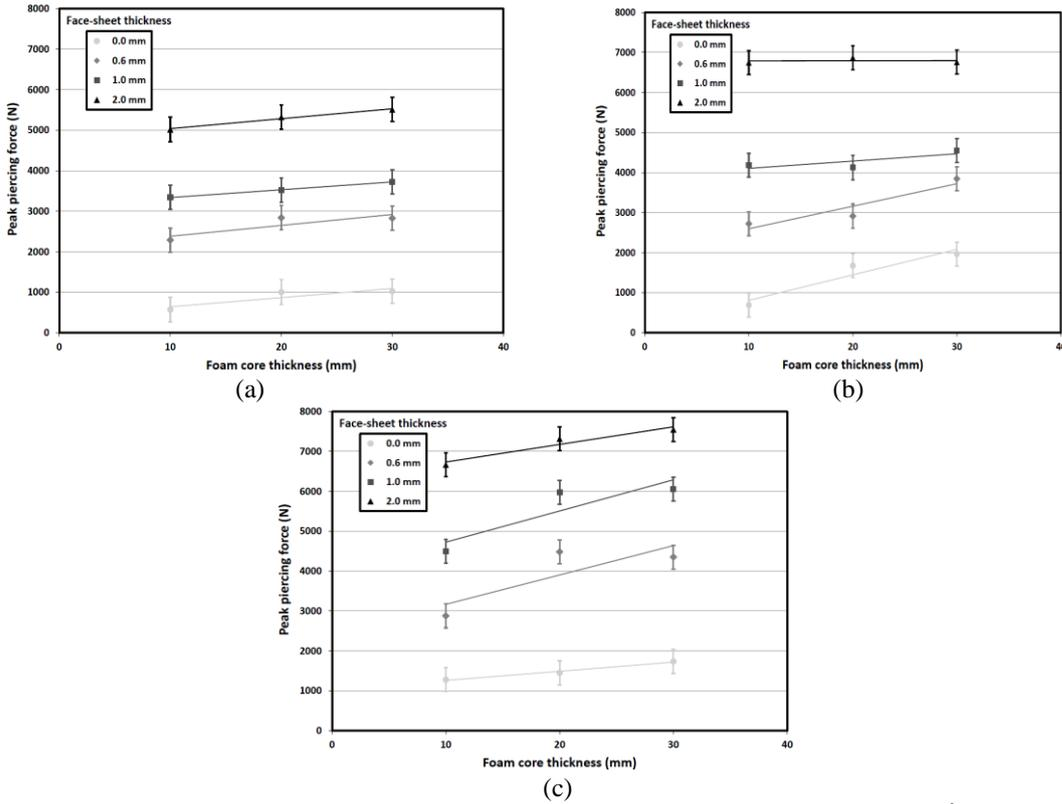
Fig. 8. Effect of foam core thickness on peak piercing force of a) 0.5 g/cm<sup>3</sup>, b) 0.6 g/cm<sup>3</sup> and c) 0.7 g/cm<sup>3</sup> foam core density specimens
