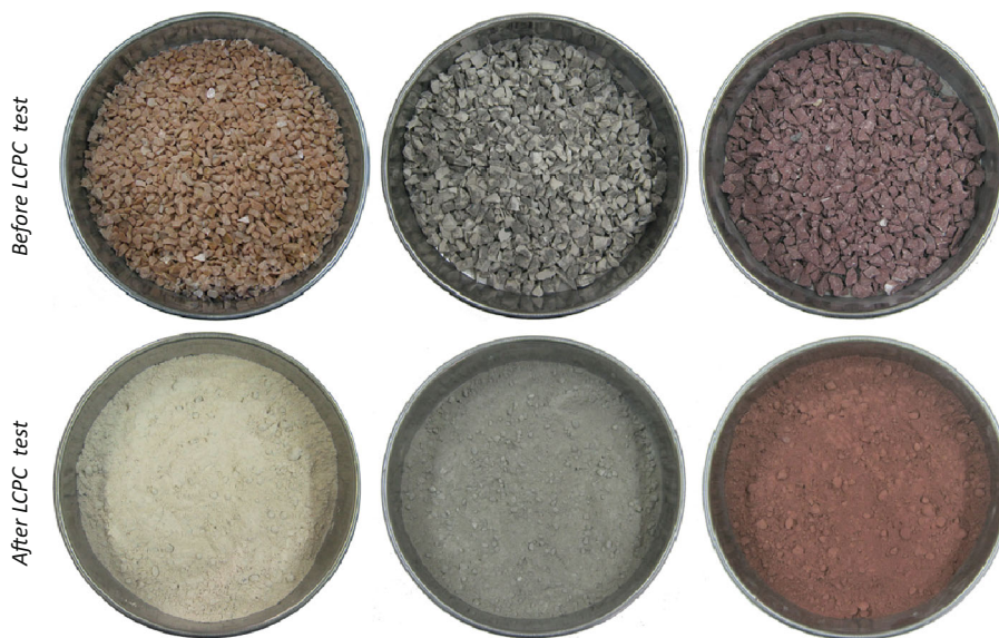
Fig. 2 A number of samples ready for testing (left to right: orthoclase, limestone and sandstone); sieve diameters are 21 cm
