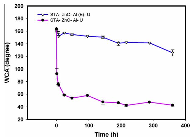
Fig. 10. Long-term stability of STA-ZnO-Al-U and STA-ZnO-Al(E)-U in NaCl solution (3.5%).
