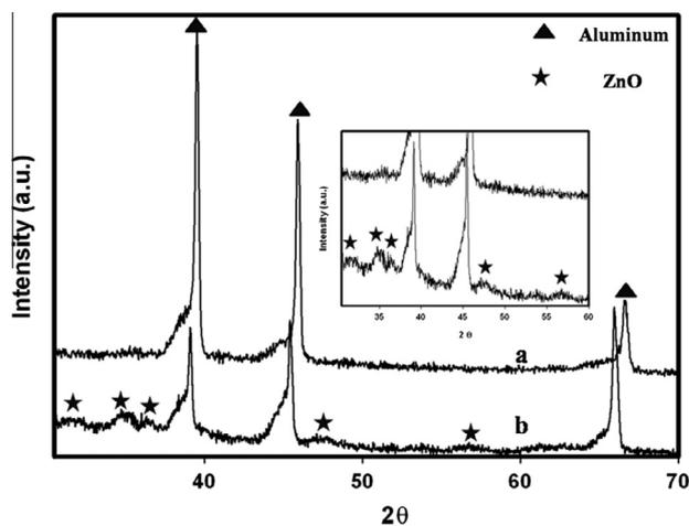
Fig. 7. XRD spectra of (a) ZnO-Al-I and (b) ZnO-Al-U.
