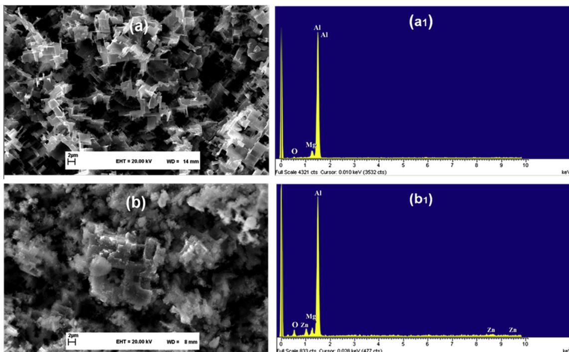
Fig. 6. SEM images (left) and EDX spectra (right) of Al(E) (a and a<sub>1</sub>) and ZnO-Al(E)-U (b and b<sub>1</sub>).
