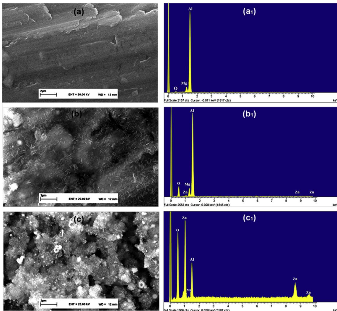
Fig. 5. SEM images (left) and EDX spectra (right) of B. Al (a and a<sub>1</sub>), ZnO–Al–I (b and b<sub>1</sub>) and ZnO–Al–U (c and c<sub>1</sub>) methods.
