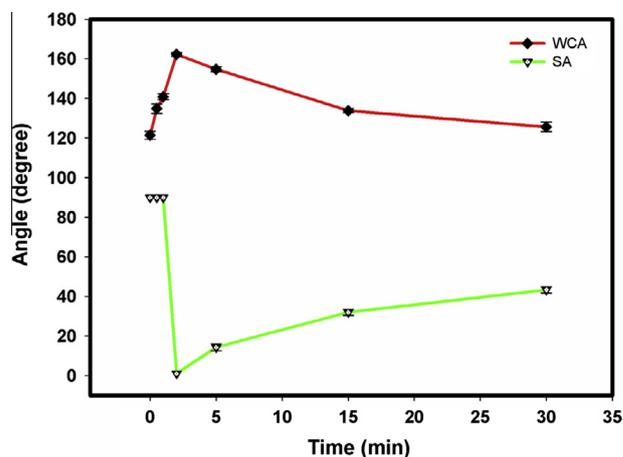
Fig. 4. WCA and SA versus time of sonication in  $\text{Zn}(\text{AC})_2$ -TEA solution.
