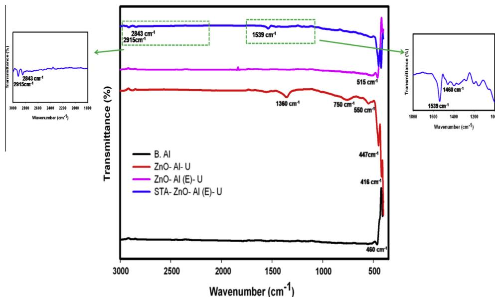
Fig. 8. ATR-FTIR spectra of different substrates.
