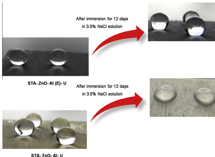
Fig. 11. Water droplet images on M.E.Z. Al and M.Z. Al. US surfaces after long-term stability test in 3.5% NaCl solution for 12 days.
