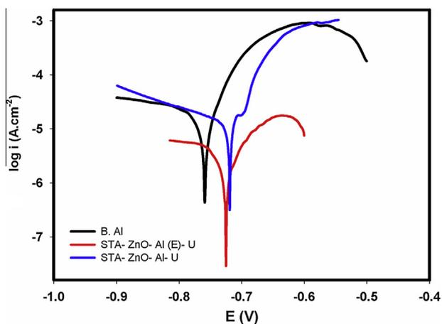
Fig. 9. Potentiodynamic polarization curves of B. Al, STA-ZnO-Al-U and STA-ZnO-Al(E)-U substrates.
