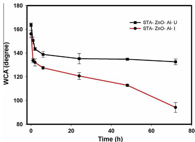
Fig. 3. WCA of STA-ZnO-Al-U and STA-ZnO-Al-I versus immersion time in water.
