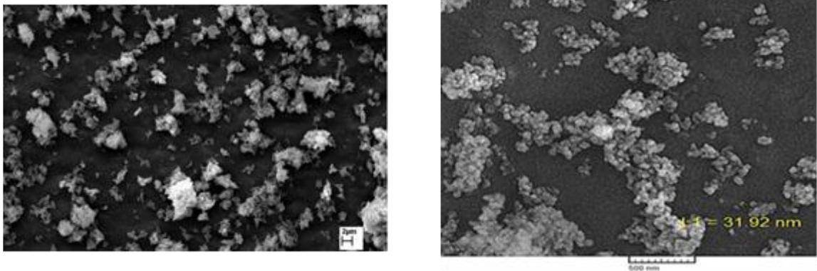
Fig. 1. SEM micrographs of starting powders (a)  $\text{CaCO}_3$ ; (b) Nano particles of  $\text{Al}_2\text{O}_3$ .
