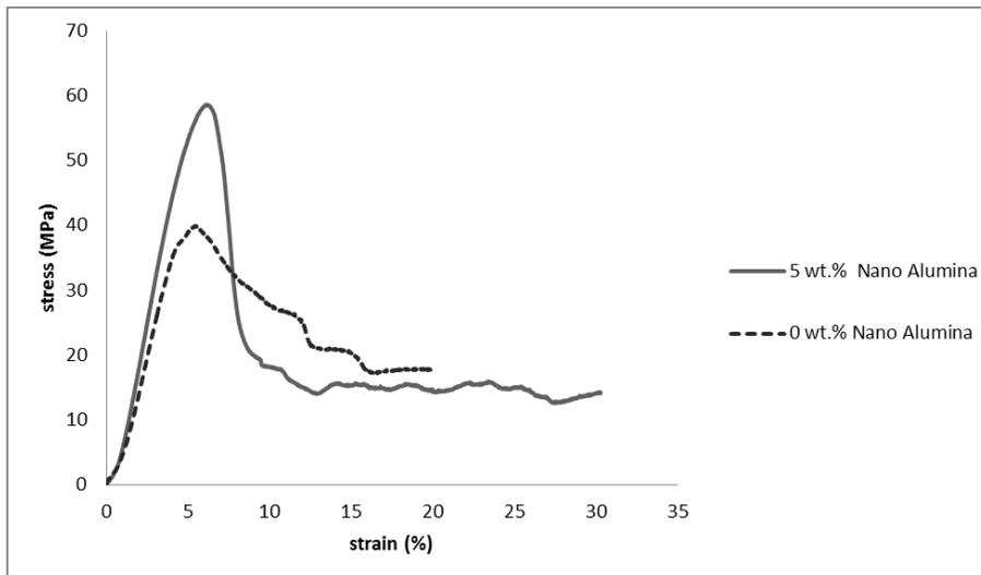
Fig.4. Compressive behavior of pure Al foam and Al- 5 wt.% Alumina Nano composite foam with about 40 % porosity.
