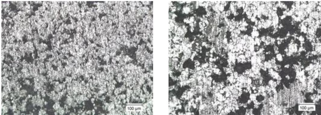
Fig. 2. Microstructure of Al- foams (a) without Al<sub>2</sub>O<sub>3</sub>; (b) with 5 wt. % Nano particles of Al<sub>2</sub>O<sub>3</sub>.
