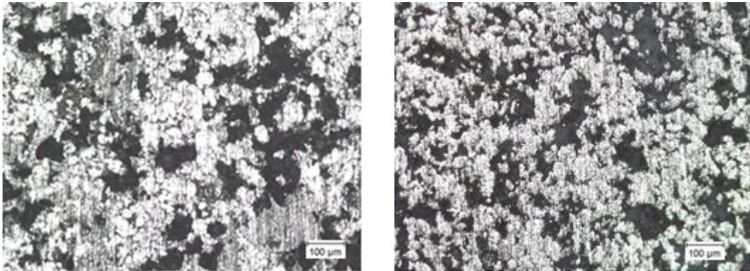
Fig.3. Optical microscopic images of nano composite Al- foams with (a) 10 wt. %  $\text{CaCO}_3$  ; (b) 15 wt. %  $\text{CaCO}_3$ .
