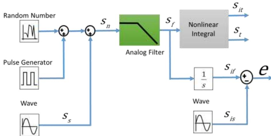
Fig. 2. Simulink environment for modeling the nonlinear integrator
