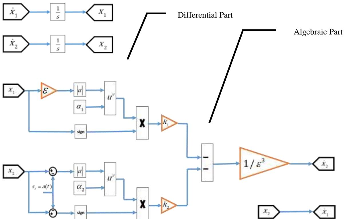
Fig. 3. Schematic of simulink environment for implementing nonlinear integrator using differential-algebraic
