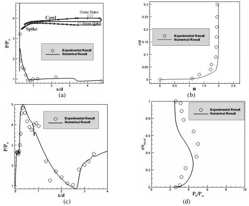
Fig. 5. Comparison of the Numerical and Experimental Data for Validation Intake at  $M_{\infty}$ =2.0 [16, 18], a) Static Pressure Ratio Distribution on the Cowl, b) Mach Number Distribution from the Outer Rake (*r* is measured from the local wall), c) Static Pressure Ratio Distribution on the Spike, d) Total Pressure Distribution from the Inner Rake (*r* is measured from the local wall), e) Shock Structures
