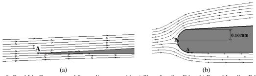
Fig. 8. Cowl Lip Geometry and Streamlines around it, a) Sharp Leading Edge, b) Round Leading Edge
