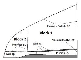
Fig. 2. Computational blocks and boundary conditions used in the numerical code
