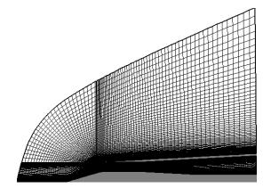
Fig. 3. The Structured Grid Inside and Around the Intake
