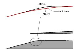
Fig. 10. Two Surface Fillets Upstream of the Throat
