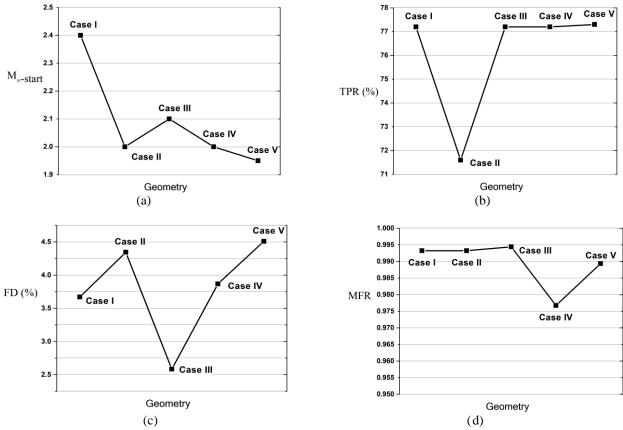
Fig. 12. Starting mach number and intake performance for various geometries, a) Free stream starting Mach number, b) TPR, c) FD, d) MFR
