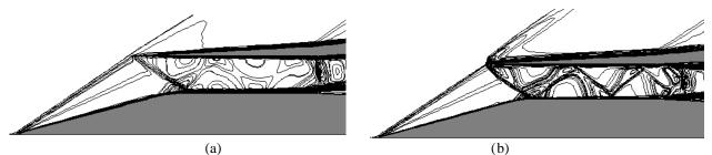
Fig. 13. Contours of Mach number at  $M_{\infty}$ =2.00 at Critical Condition, a) Case II, b) Case III
