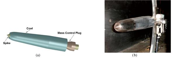
Fig. 4. Intake Used for the Code Validation [18], a) Schematic View, b) Mounted in the Test Section
