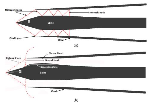
Fig. 1. Intake Geometry and Shock Pattern, a) at Start (Design) Condition, b) at Unstart Condition
