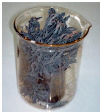
Fig. 1. (Color online) Tree-like structure (dendritic structure) of strontium hexaferrite powders after auto-combustion and before any annealing treatment.
