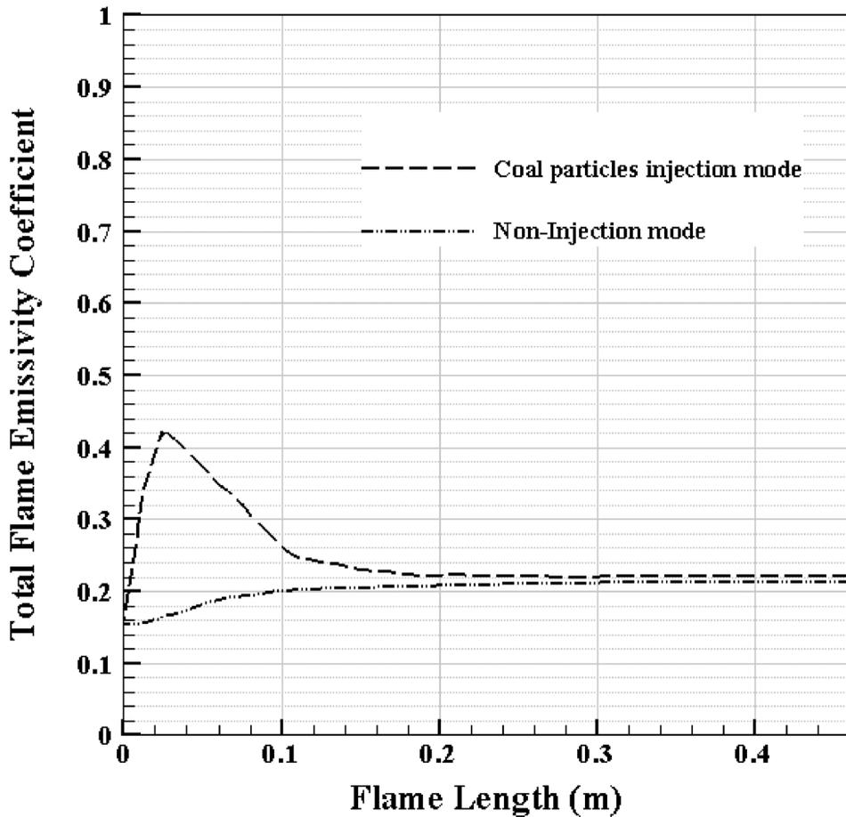
Fig. 7. Total emissivity coefficient of flame considering the radiation of soot particles for injection and noninjection modes.
