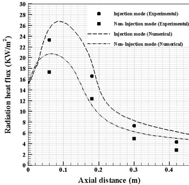
Fig. 3. Axial radiation heat flux along the furnace centerline for injection and noninjection modes (Experiment from Ref. 17).
