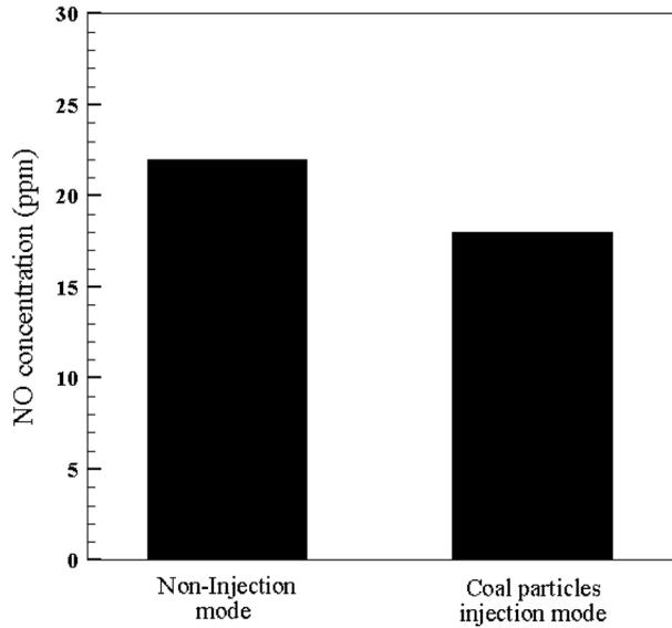
Fig. 9. NO pollutant emission in injection and noninjection modes.
