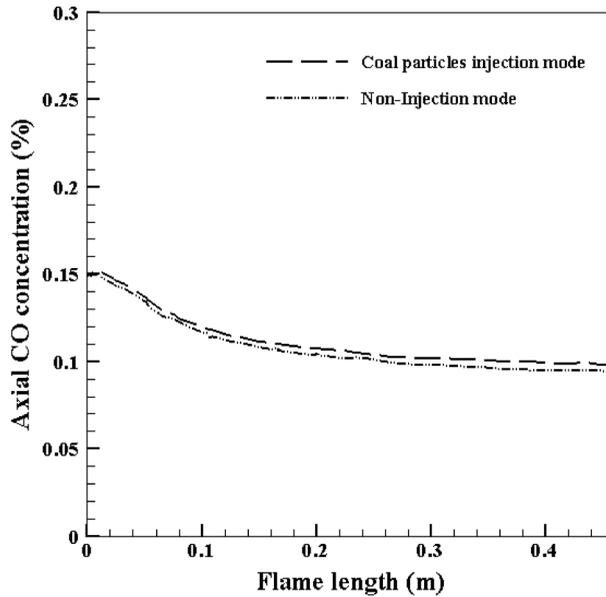
Fig. 8. CO concentration across the furnace axis for injection and noninjection modes.
