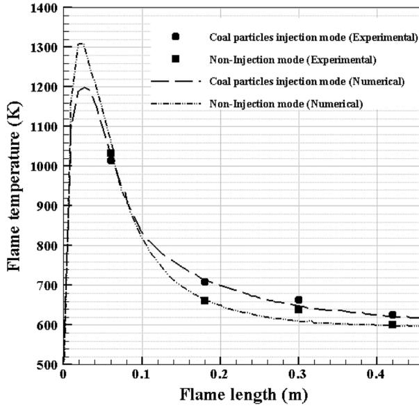
Fig. 2. Temperature distribution along the furnace centerline for injection and noninjection modes (Experiment from Ref. 17).
