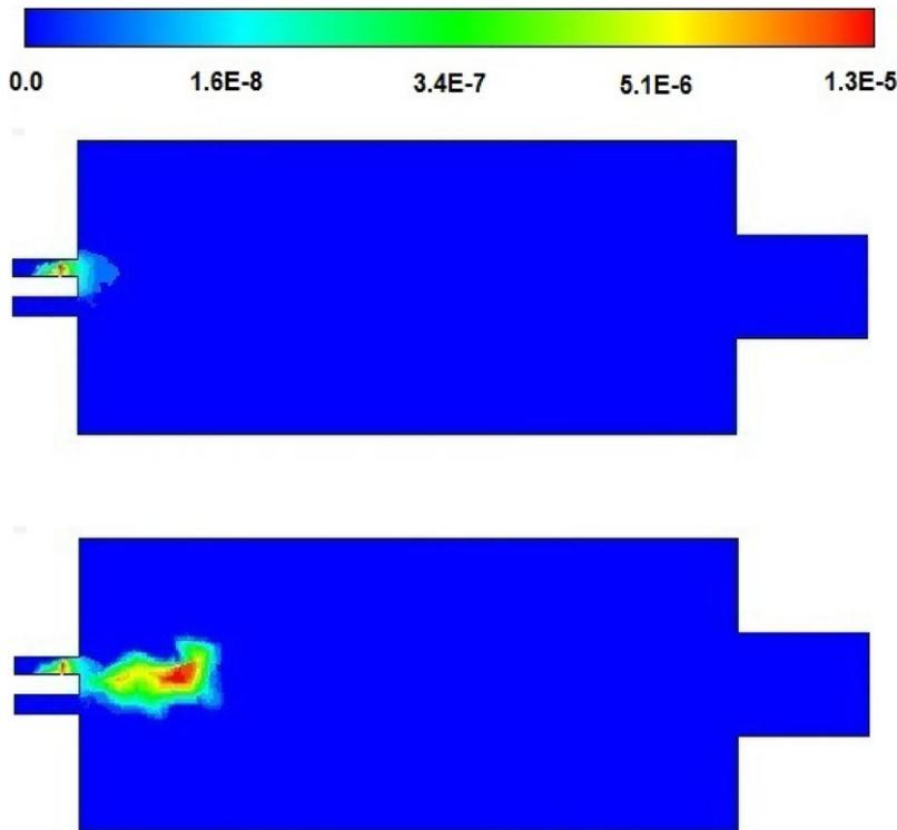
Fig. 6. Soot particles distribution within the furnace for noninjection (top) and injection (bottom) modes. [Color figure can be viewed in the online issue, which is available at [wileyonlinelibrary.com/journal/htj](http://wileyonlinelibrary.com/journal/htj).]
