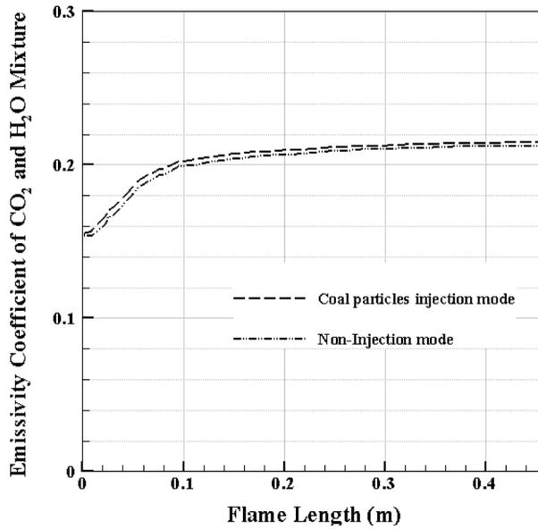
Fig. 4. Emissivity coefficient of the  $\text{CO}_2$  and  $\text{H}_2\text{O}$  gas mixture along the furnace centerline for injection and noninjection modes.
