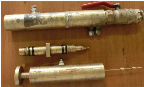
Fig. 9. A photograph of variable geometry ejector.
