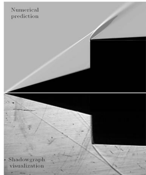
Figure 5. Comparison of numerical axial density gradient contour with experimental shadowgraph image, M_\infty = 2.0 and \alpha = 0 .
