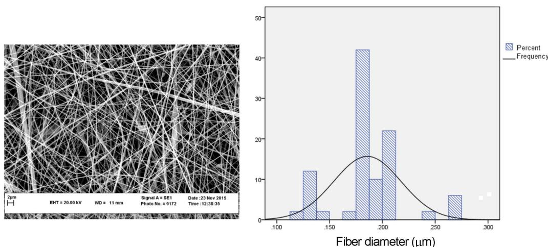
**Figure 10.** SEM image and fiber diameter distribution of zein fibers electrospun at optimized condition.
