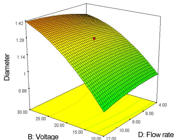
**Figure 6.** Influence of solution flow rate (ml/h) on fiber diameter ( $\mu\text{m}$ ) in electrospinning at a constant zein solution concentration of 26 w/v %, and distance between needle tip and collector of 15 cm.
