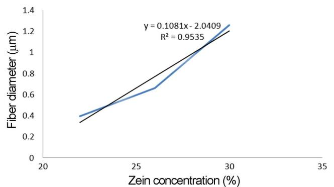
Figure 4. Effect of zein concentration (w/v %) on diameter (μm) of zein fibers electrospun at a constant applied voltage of 20 kV, flow rate of 8 ml/h and distance between needle tip and collector of 15 cm.
