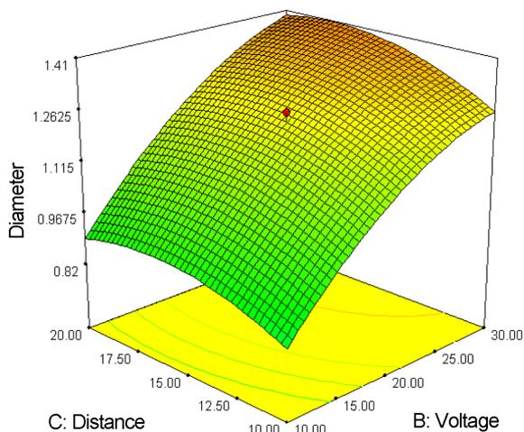
**Figure 5.** Influence of applied voltage (kV) on fiber diameter ( $\mu\text{m}$ ) in electrospinning at a constant zein solution concentration of 26 w/v %, flow rate of 8 ml/h.
