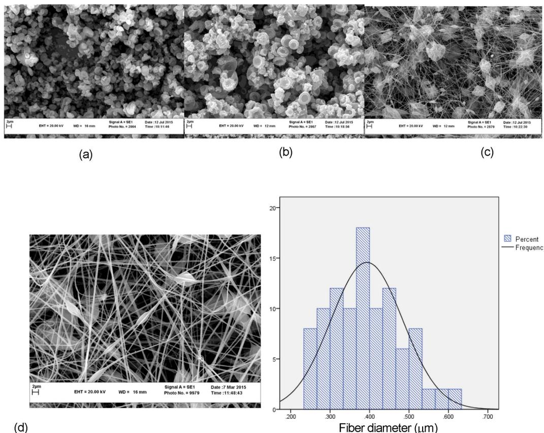
**Figure 2.** SEM images of zein fibers electrospun at a constant applied voltage of 20 kV, flow rate of 8 ml/h, and distance between needle tip and collector of 15 cm and at various zein concentrations; (a) 10 w/v %, (b) 15 w/v %, (c) 20 w/v %, (d) 22 w/v %, (e) 26 w/v %, and (f) 30 w/v %.
