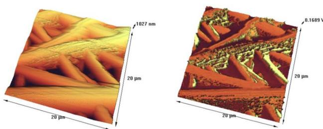
Figure 3. AFM 3D-topograph (left) and amplitude (right) images of zein fibers electrospun at a constant concentration of 26 w/v %, applied voltage of 20 kV, flow rate of 8 ml/h, and distance between needle tip and collector of 15 cm.
