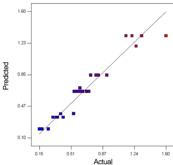
**Figure 8.** The predicted versus actual plot for average fiber diameter of electrospun zein fiber.
