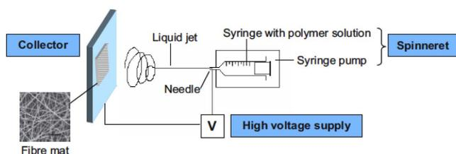
Figure 1. Schematic of the electrospinning unit.
