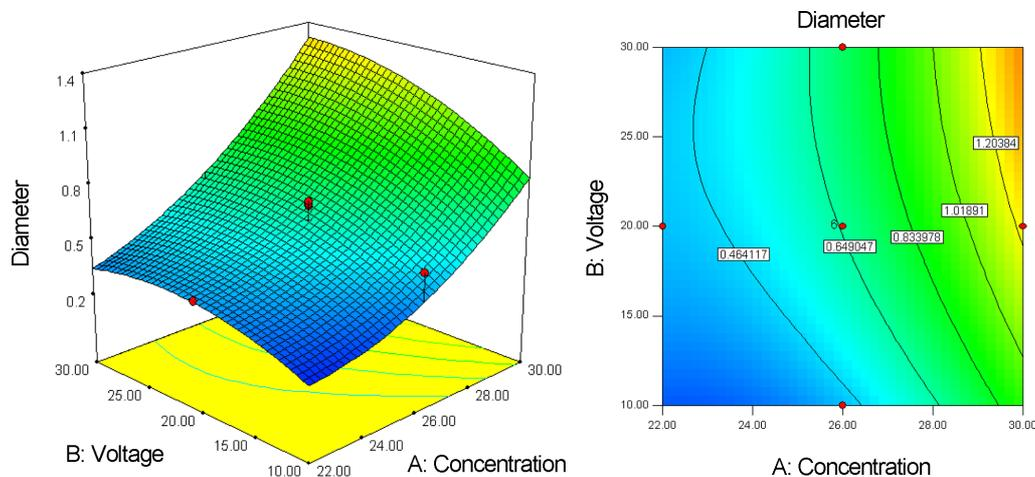
**Figure 9.** Response surface and contour plots of fiber diameter ( $\mu\text{m}$ ) showing the effect of solution concentration (w/v %) and applied voltage (kV).
