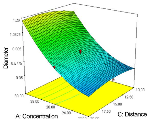
**Figure 7.** Influence of distance between needle tip and collector (cm) on fiber diameter ( $\mu\text{m}$ ) in electrospinning at applied voltage of 20 kV and flow rate of 8 ml/h.
