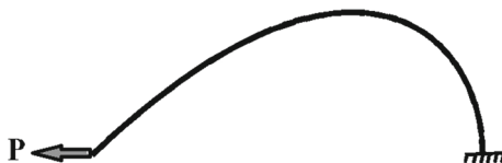
Fig. 14 The configuration of a Tschirnhausen cantilever beam used in Example 4
