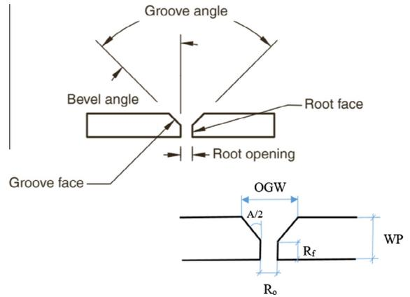
Fig. 2. Joint edge specifications for GMAW of plates with more than 6 mm thickness.
