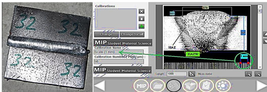
Fig. 5. Quantitative evaluation of WBG and HAZ using microstructural image processing software.
