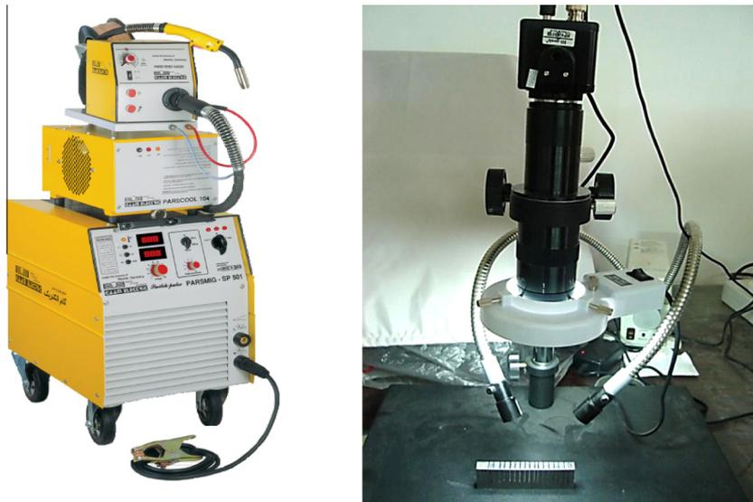
Fig. 4. GMAW machine and optical microscope used.
