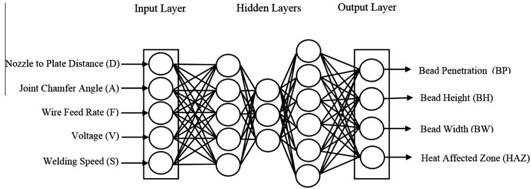
Fig. 6. Architecture of proposed BPNN model.
