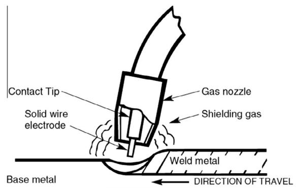
Fig. 1. A schematic representation of GMAW process.
