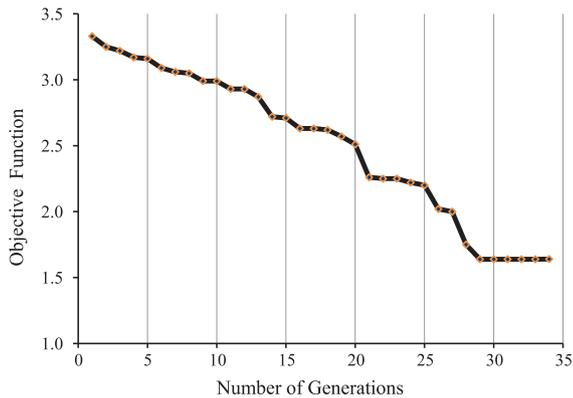
**Fig. 9.** Convergence curve for the proposed PSO algorithm.
