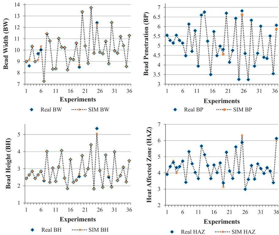
Fig. 7. Comparison between experimental and predicted BW, BP, BH and HAZ by the BPNN models.
