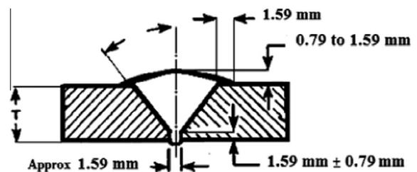
Fig. 8. Desirable V-beveled butt joint for gas pipeline and related facilities [19].
