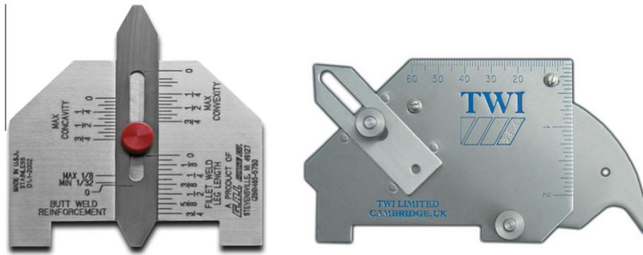
Fig. 3. Bridge Cam and AWS gauges used to measure BHs and BWs of the welded specimens.
