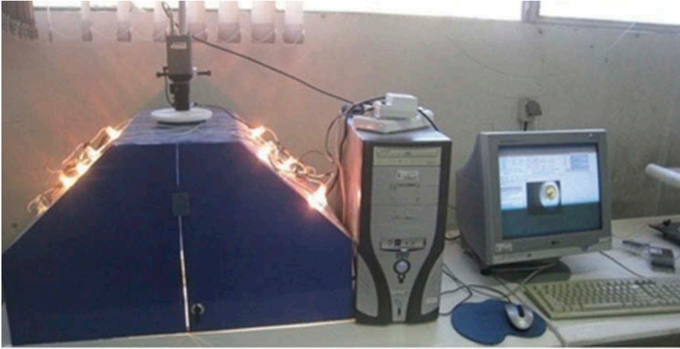
Figure 2. The constructed multispectral imaging system for acquiring images from the fruit.
