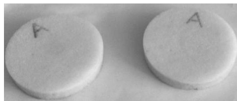
Fig. 1 Samples of sound absorption coefficient test
