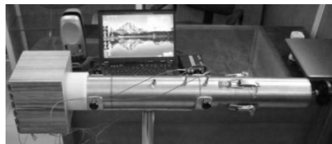
Fig. 2 Impedance tube used in this investigation
