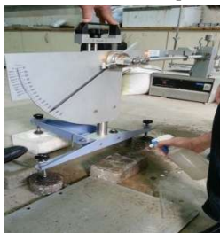
Figure 9 - Sprinkle CMA solution on samples
