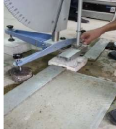
Figure 6 - placing the concrete samples in device of British Pendulum
