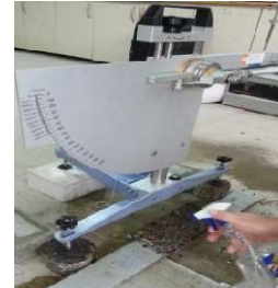
Figure 8 - Sprinkle salt solution on samples
