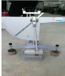
Figure 7 - placing the self-compacting concrete samples in device of British Pendulum
