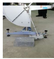
Figure 3 - View of the British pendulum device (pendulum friction) in the pavement laboratory
