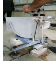
Figure 4 - placing the aggregates samples in device of British Pendulum
