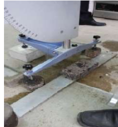
Figure 5 - placing the Asphalt samples in device of British Pendulum
