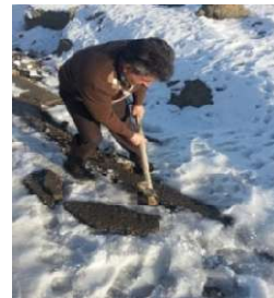
Figure 1 - Preparation of asphalt samples by digging the road surface
