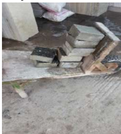
Figure 2 - Concrete samples which were cut in stone cutting factory
