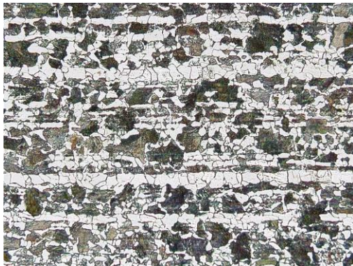
Figure 3 - grain orientation of rolled steel.
