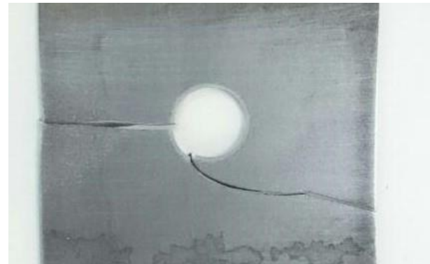
Figure 5 - fatigue crack path in the specimen with circular cutout
