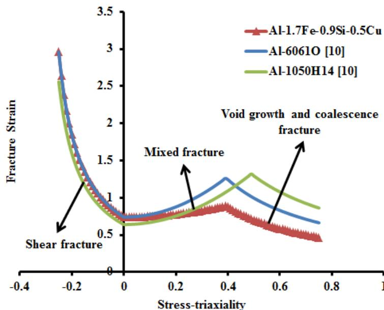
Figure 6: Comparison of fracture strain vs. stress-triaxiality curve for different aluminum alloys.
