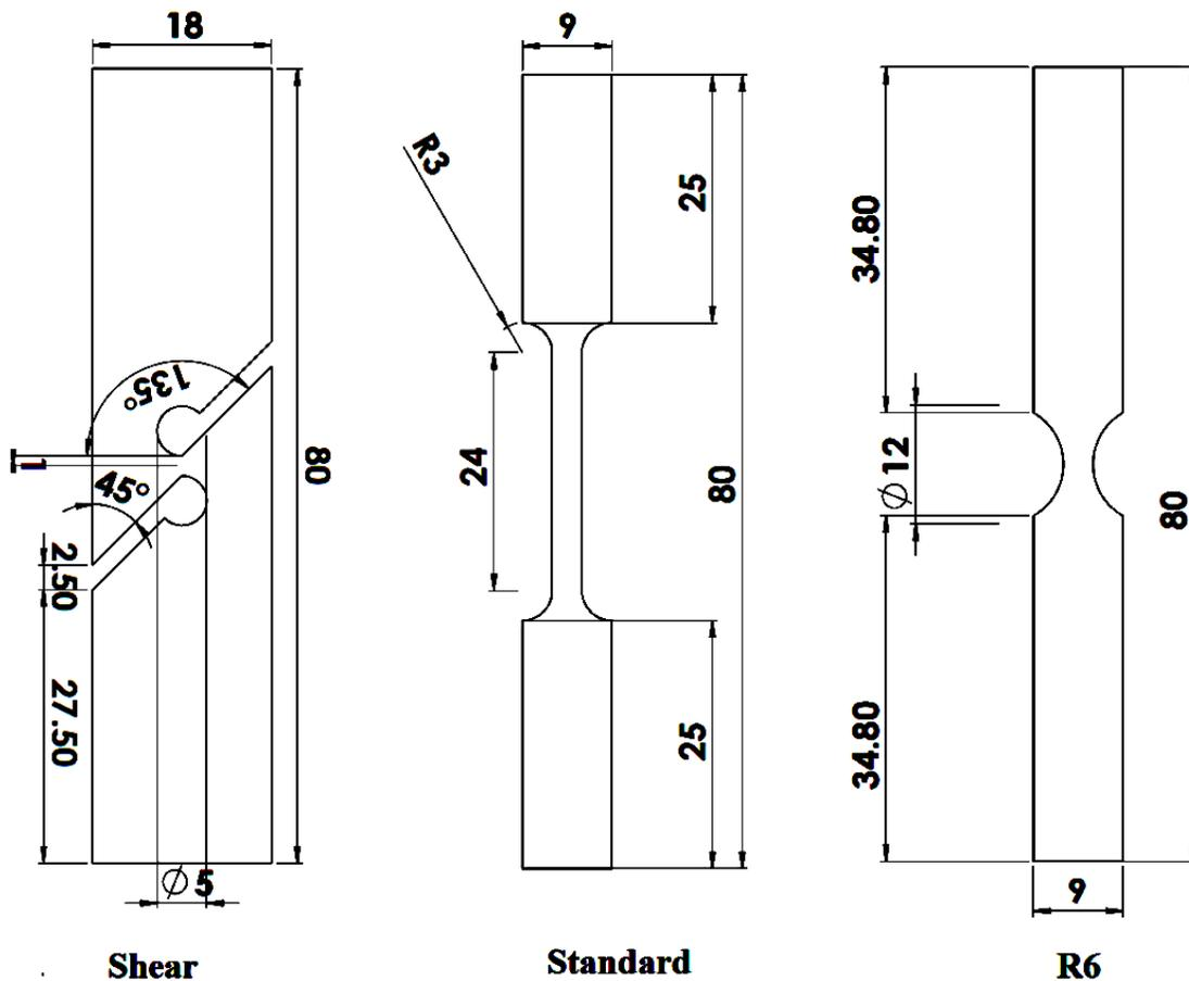
Figure 1: Geometry and dimensions of tensile specimens.
