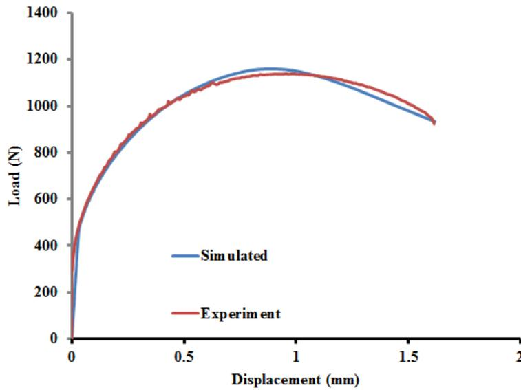
Figure 3: Experimental and simulation results for load-displacement of R6 tensile test.
