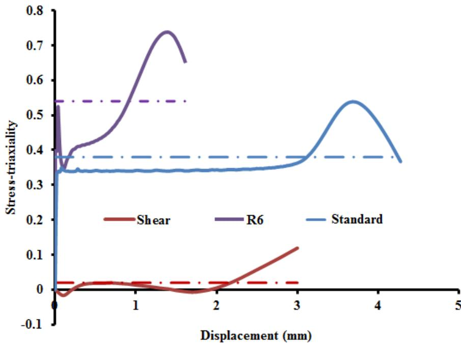
Figure 4: Variation of stress-triaxiality by displacement for different specimens.
