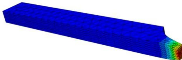
Figure 5: Distribution of equivalent plastic strain at  $\Delta L_f$  for: (a) Standard, (b) shear and (c) R6.
