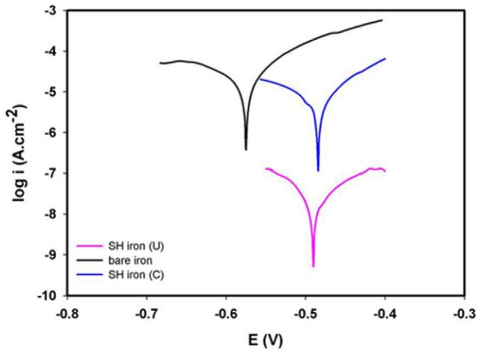
Fig. 6. Potentiodynamic polarization curves for bare iron, SH iron (U) and SH iron (C).
