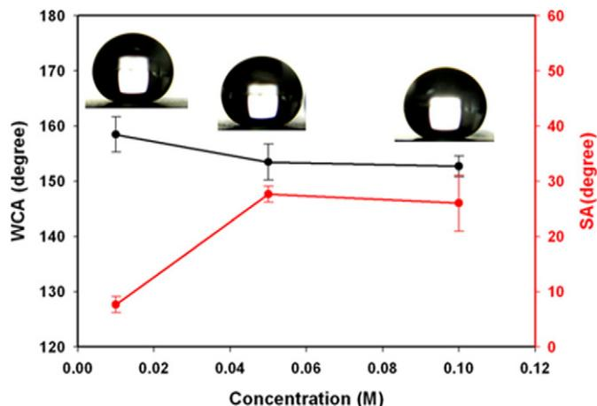
**Fig. 3.** WCA and SA versus starting material concentration.
