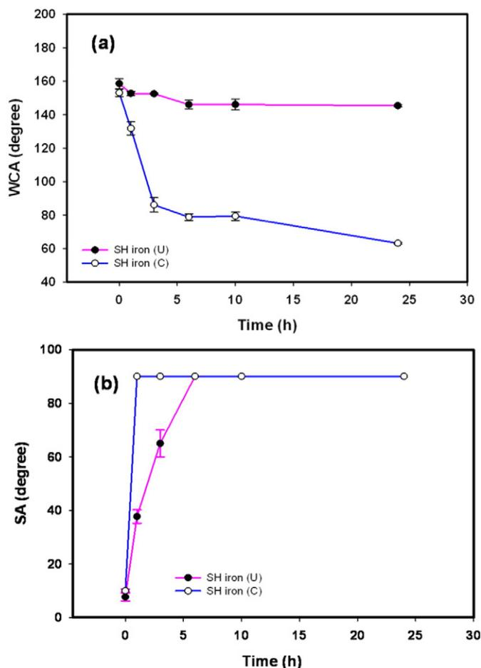
**Fig. 4.** a) WCA and b) SA values versus time immersion in NaCl solution (3.5%).
