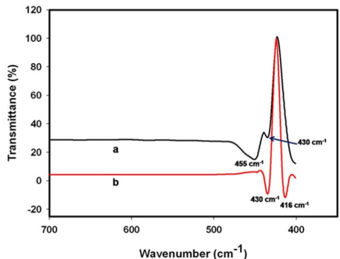
Fig. 10. ATR-FTIR spectra of a) bare iron and b) ZnO-iron-U surface.
