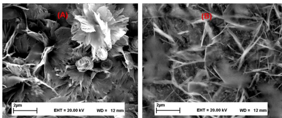
**Fig. 5.** SEM images of SH iron (U), A) before and B) after immersion in NaCl solution (3.5%) for 3 h.
