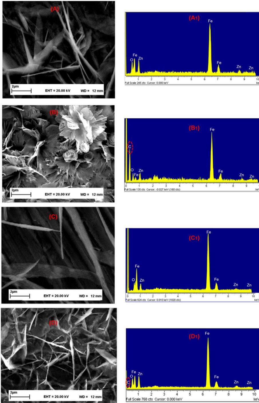
Fig. 11. SEM images (left) and EDX spectra (right) of (A, A<sub>1</sub>) ZnO-iron-U, (B, B<sub>1</sub>) SH iron (U), (C, C<sub>1</sub>) ZnO-iron-C and (D, D<sub>1</sub>) SH iron (C).
