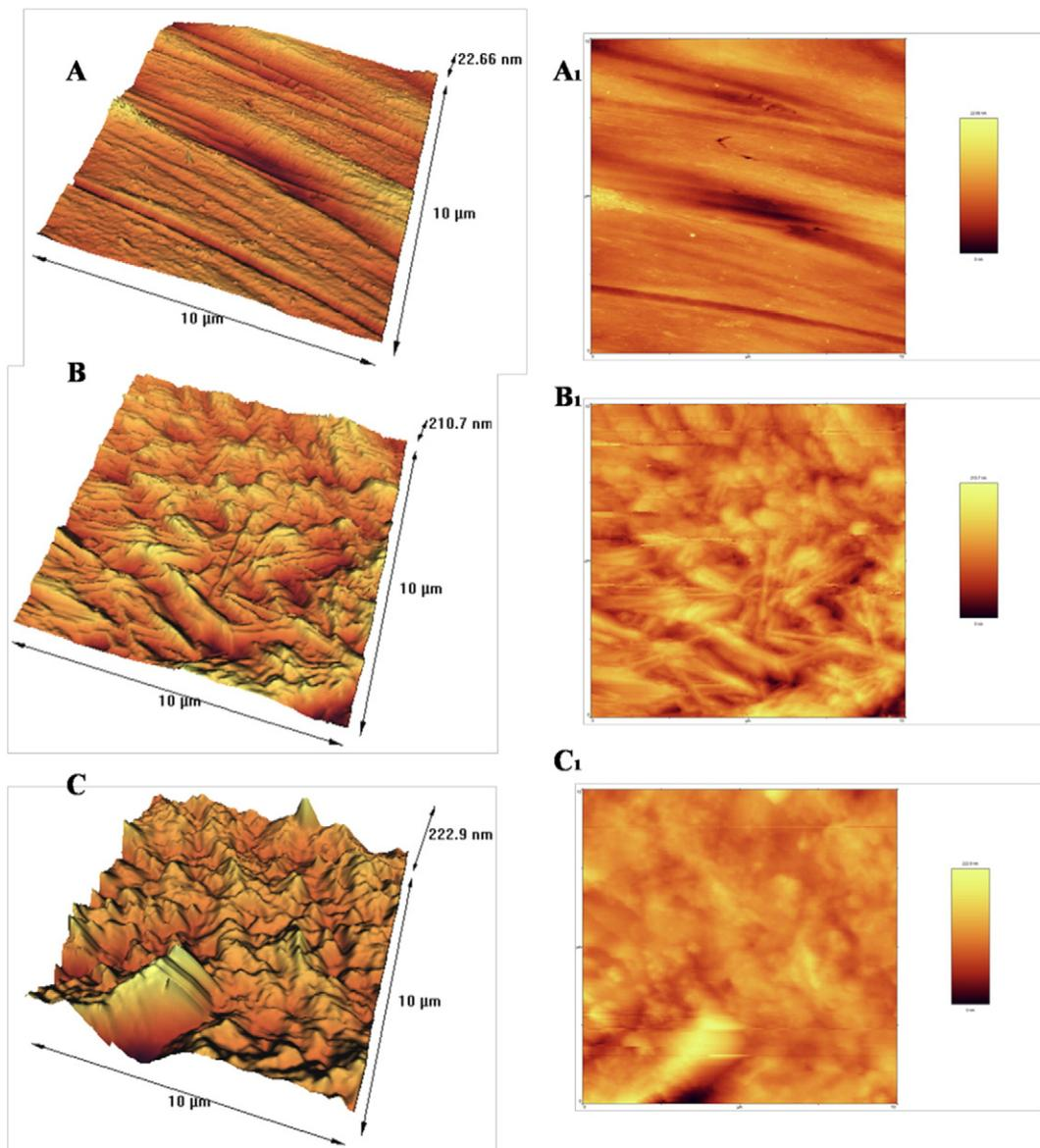
Fig. 9. 2D (right) and 3D (left) AFM images of (A, A<sub>1</sub>) bare iron, (B, B<sub>1</sub>) ZnO-iron-C and (C, C<sub>1</sub>) ZnO-iron-U.
