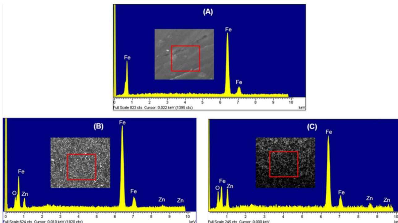
Fig. 8. EDX spectra of A) bare iron, B) ZnO-iron-C and C) ZnO-iron-U.
