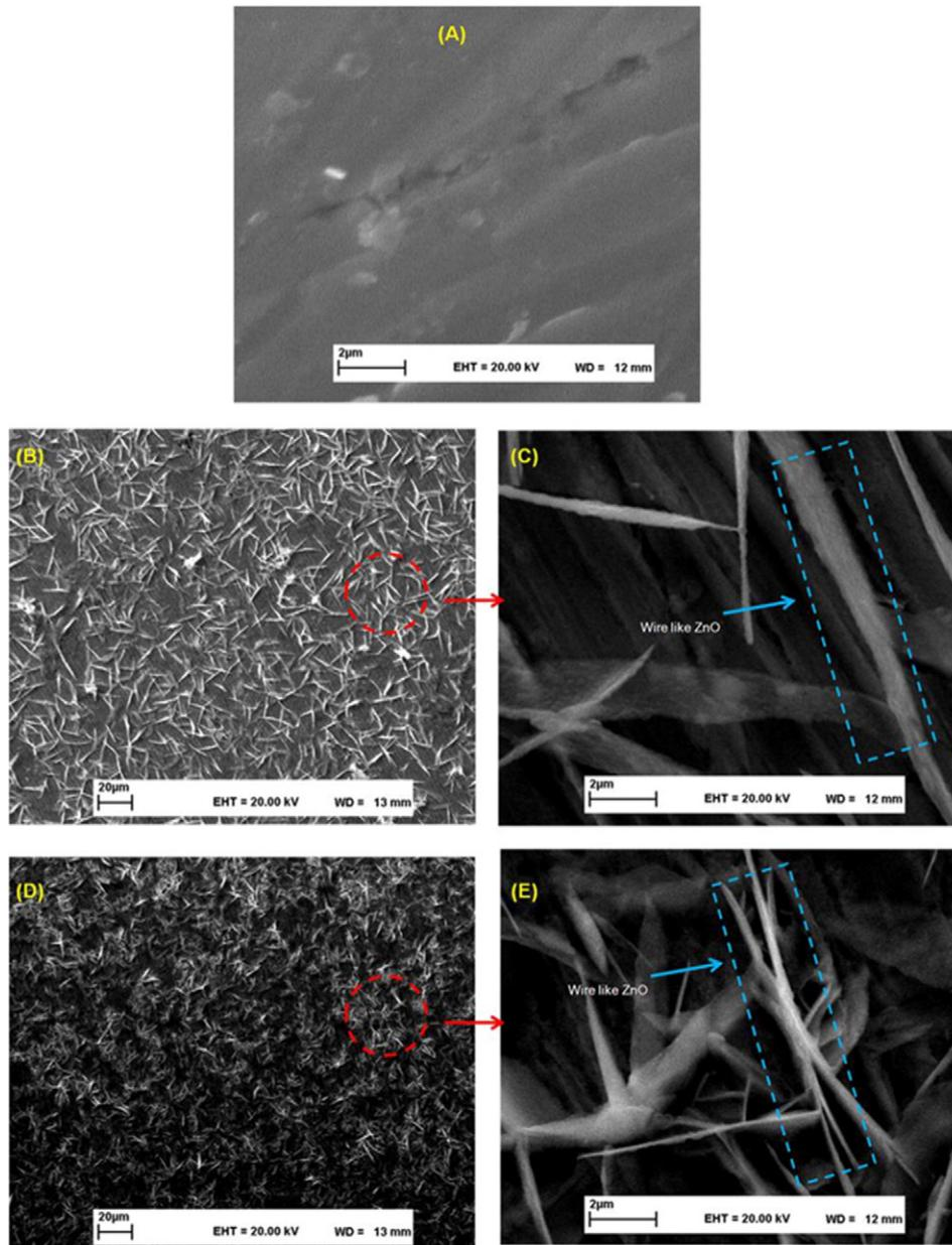
Fig. 7. SEM images of A) bare iron, B–C) ZnO-iron-C and D–E) ZnO-iron-U.
