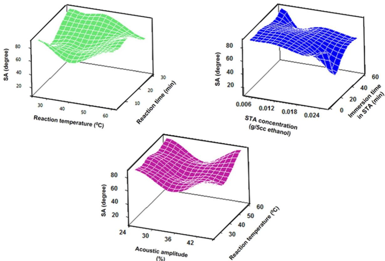
**Fig. 2.** Three-dimensional graphs of a) reaction time-reaction temperature-SA, b) STA concentration-immersion time in STA-SA and c) acoustic amplitude-reaction temperature-SA.
