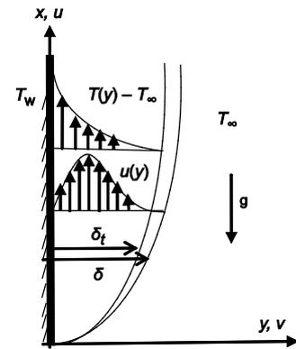
Figure 1. Laminar boundary layer on a hot vertical flat plate in free convection
