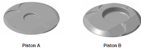
Fig. 2.Geometry of the combustion chambers on pistons
