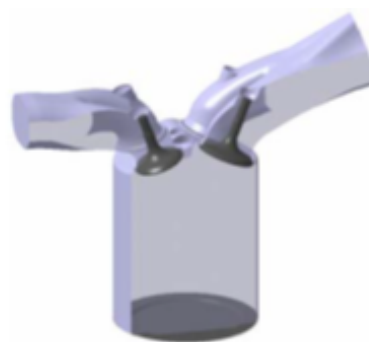
Figure 1. Schematic view of typical engine model with piston crown A
