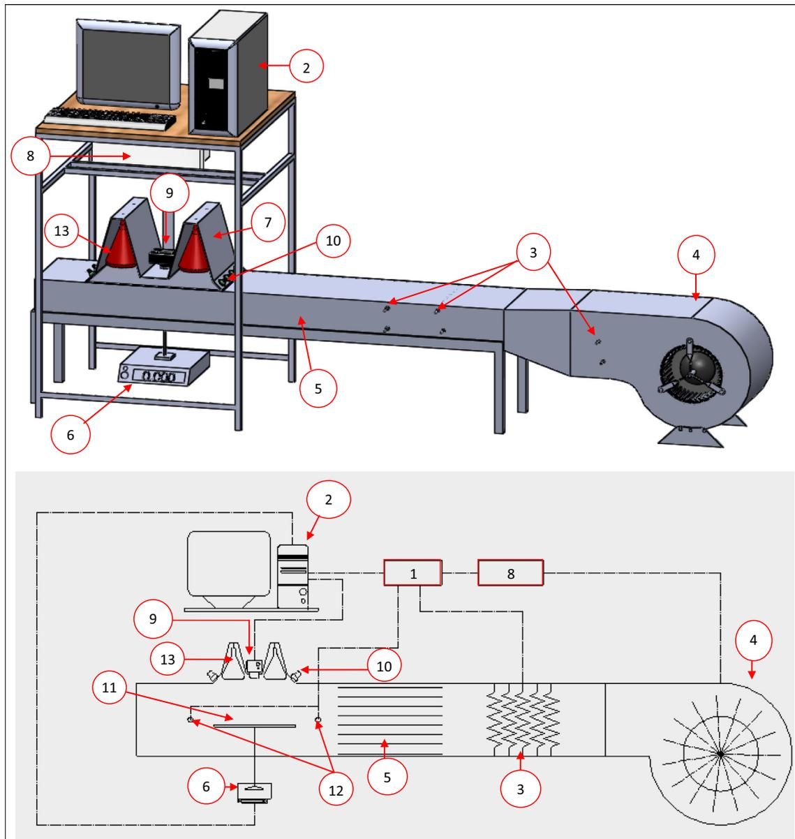
**Fig. 1.** Experimental dryer: (1) Control units; (2) PC; (3) Heating unit; (4) Fan; (5) Straightener; (6) balance; (7) Illumination and imaging chamber (a cutaway of chamber is displayed); (8) Inverter; (9) Camera; (10) Lighting lamp; (11) Tray; (12) Temperature sensors; (13) IR lamps (Nadian et al., 2016a).
