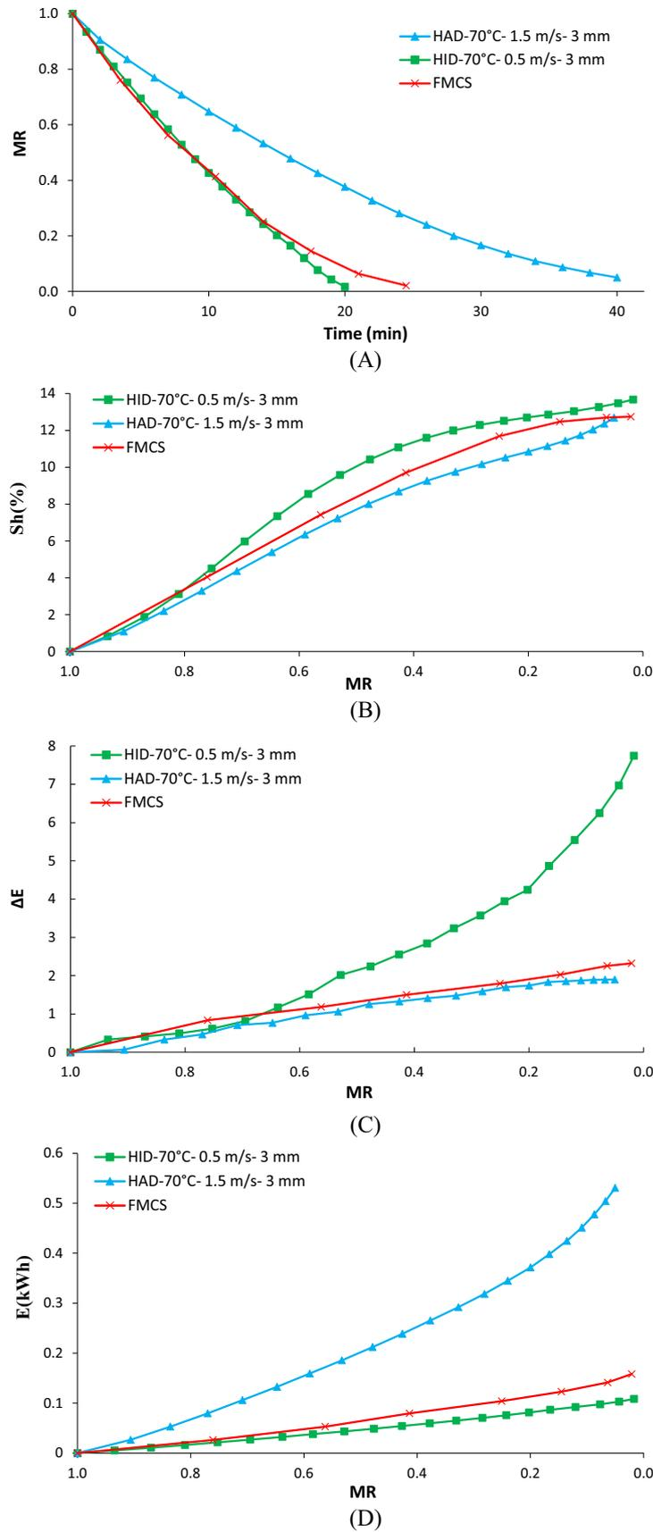
Fig. 9. Relationships between MR and drying time (A); Sh and MR (B); ΔE (color change) and MR (C); and E (Energy consumption) and MR (D) for optimal condition of HID and HAD drying methods as well as FMCS of drying.
