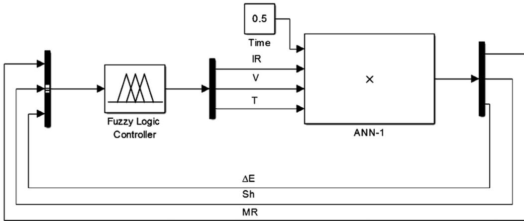
Fig. 5. Incorporating ANN-1 network to predict drying characteristics ( $\Delta E$ ,  $Sh$  and  $MR$ ) for a single chromosome in the core section of the GA code to reach the final  $MR$  (0.05).
