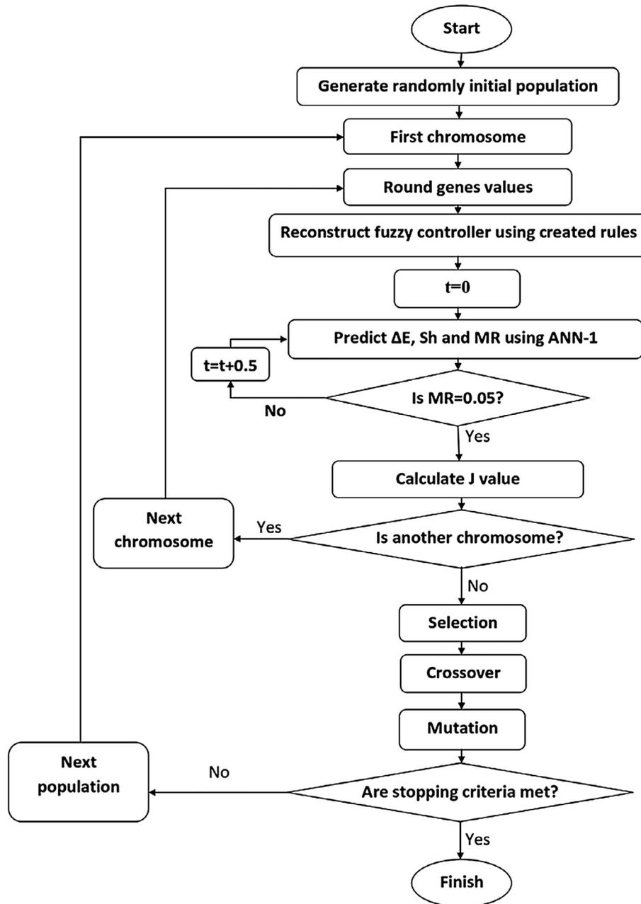
Fig. 4. The flowchart of GA optimization procedure.
