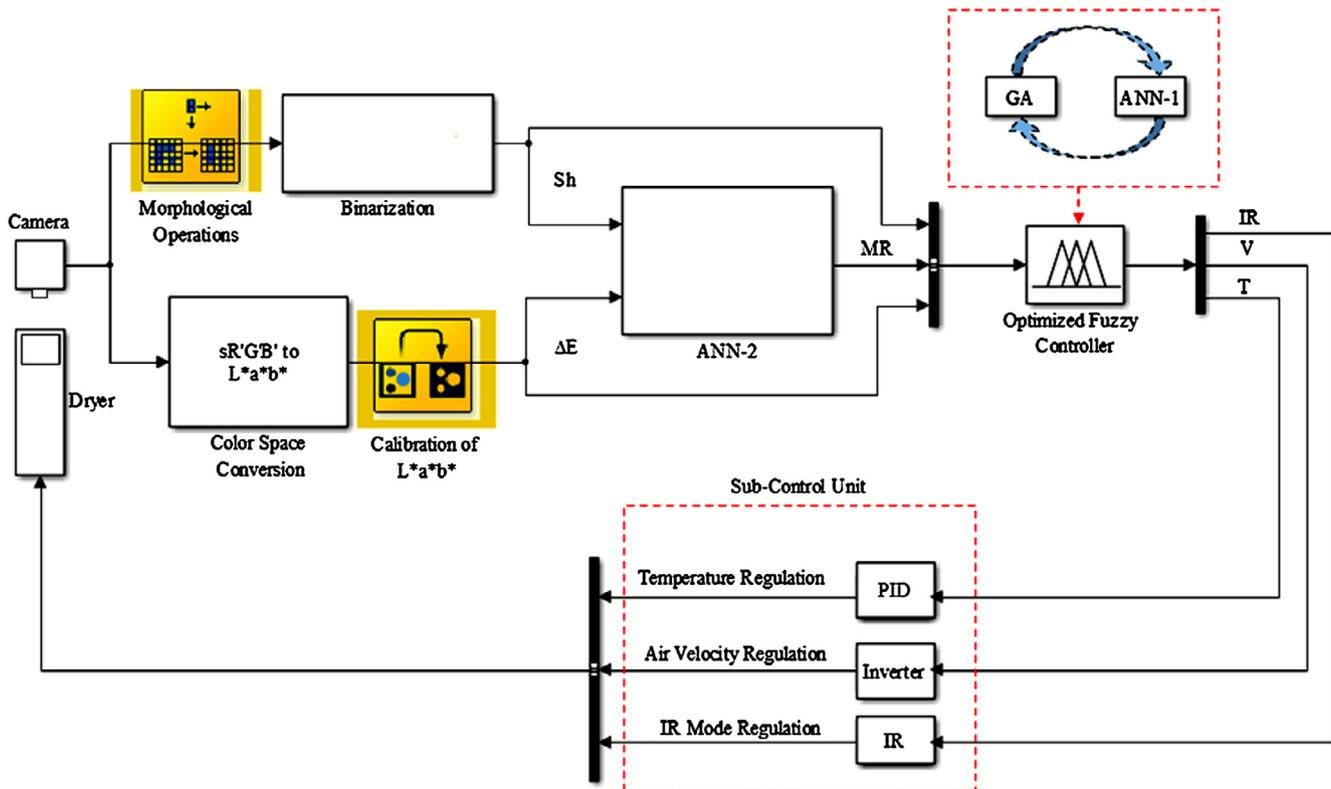
Fig. 6. The schematic diagram of the integrated control system.
