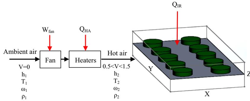
Fig. 2. Total energy flow into the control volume.
