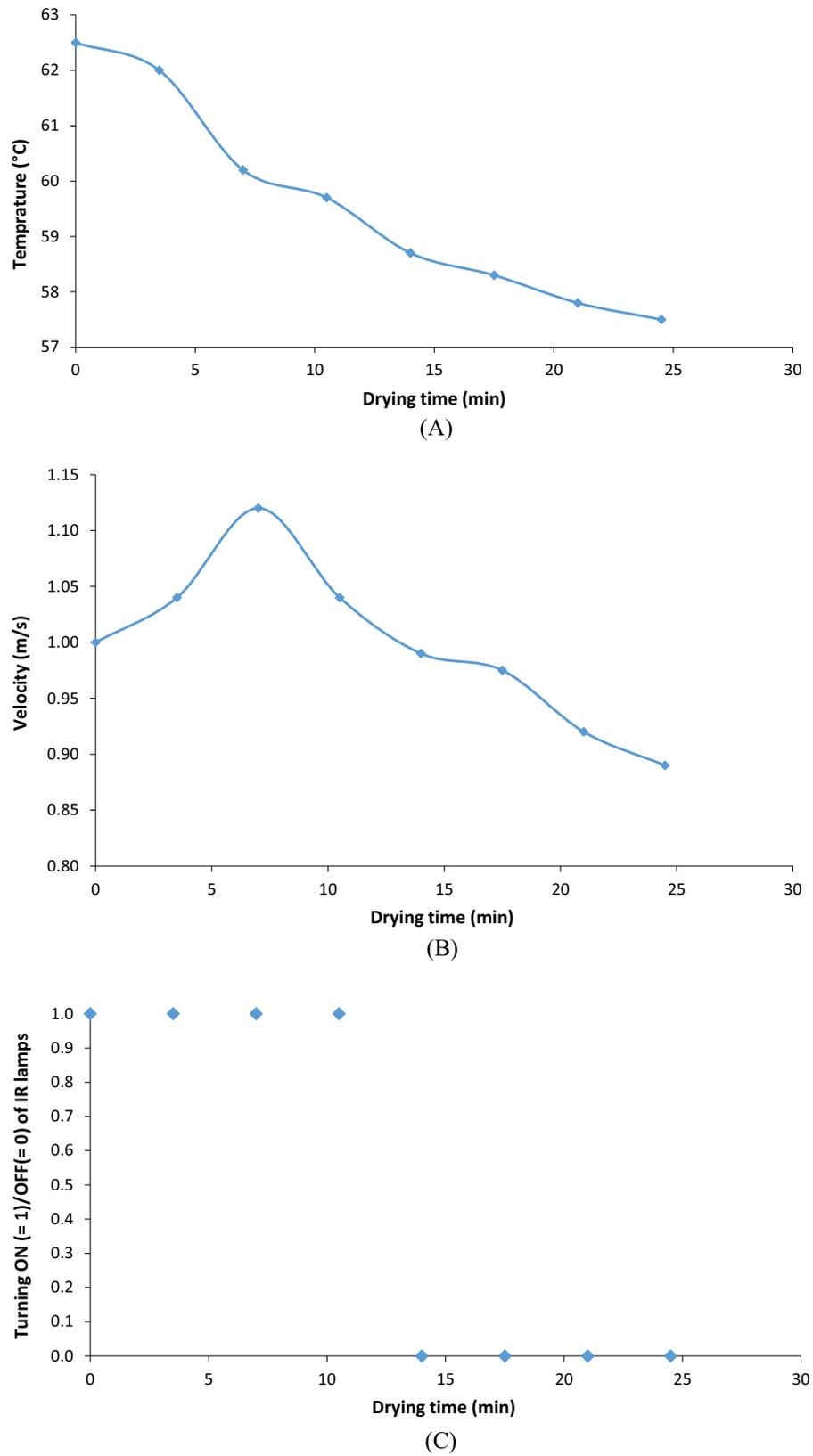
Fig. 8. Evolutions of velocity, temperature and IR mode versus drying time, during testing of FMCS.
