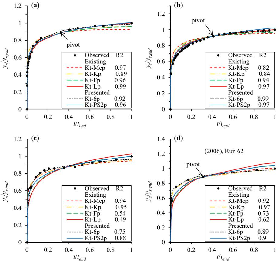
**Fig. 7** Plot of time development of SHD compared to time equations for medium-duration experiments of: **a** Shrestha (2015), run s2r6; **b** Nouri et al. (2013), run 2; **c** Amini et al. (2012), run 1–3 and **d** Ataie-Ashtiani and Beheshti (2006), run 62
