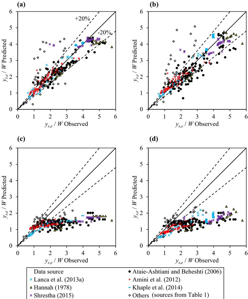
**Fig. 10** Scatter plots of predicted versus observed values of non-dimensional equilibrium scour depth for extrapolated data using equation of: **a** Present study 1 based on HEC-18; **b** present study 2 based on FDOT; **c** HEC-18 and **d** Ataie-Ashtiani and Beheshti (2006)—correction on HEC-18
