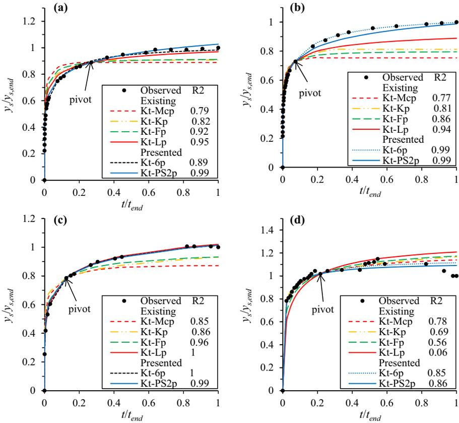
**Fig. 6** Plot of time development of SHD compared to time equations for long-duration tests of: **a** Moreno et al. (2014) run PG; **b** Lança et al. (2013a) run 3; **c** same, run 53 and **d** Smith (1999), run 7
