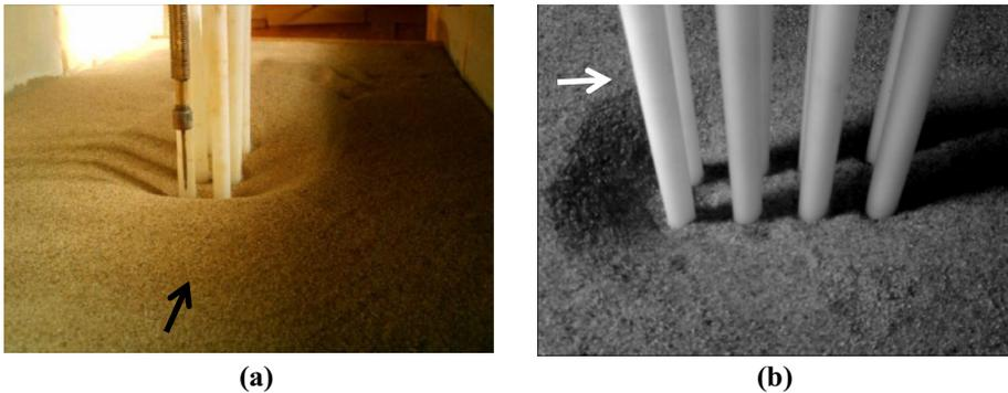
**Fig. 2** Scour hole shape around PGs after the end of the experiments and dewatering the flume with arrows showing flow direction for experiments of: **a** Baratian (2007) and **b** Hajzaman (2008)
