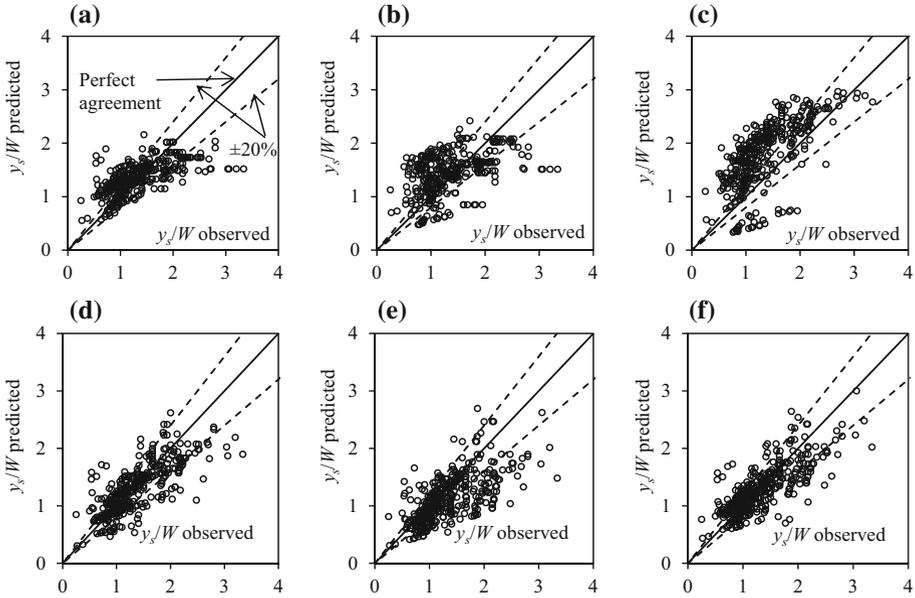
**Fig. 4** Scatter plots of predicted versus observed values of non-dimensional scour depth ( $y_s/W$ ) for raw data using equations of: **a** HEC-18, **b** Coleman (2005), **c** FDOT, **d** Ataie-Ashtiani and Beheshti (2006)—correction on HEC-18, **e** Amini et al. (2012) and **f** Beheshti et al. (2013)
