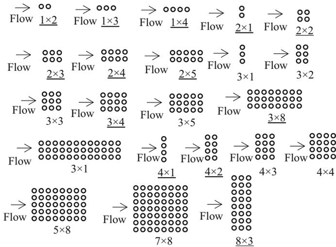
**Fig. 3** Arrangements of pile groups used in this study in the form  $n \times m$ , underlined for configurations with available time record of SHD development (in some experiments, square piles were used)
