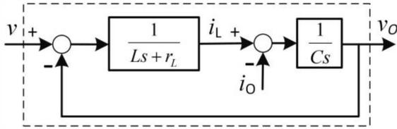
Fig. 2. Block diagram of UPS inverter
