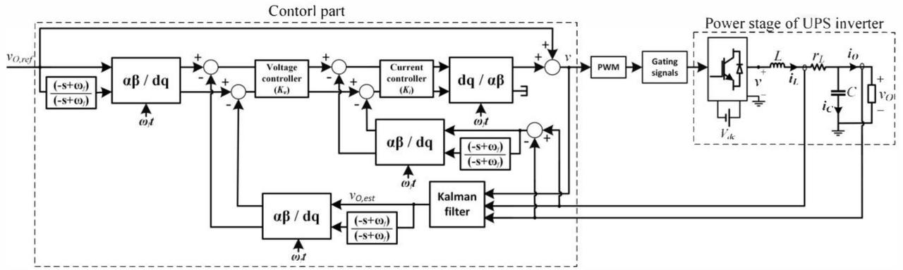
Fig. 3. Proposed control scheme for UPS inverter
