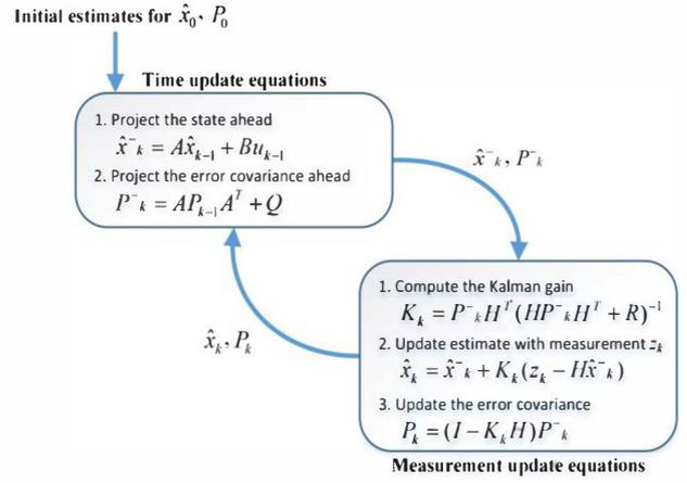
Fig. 7. Kalman filter algorithm performance
