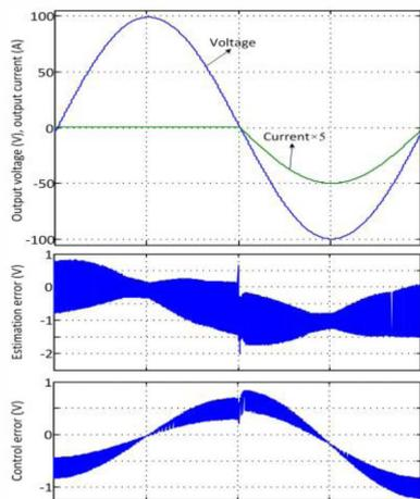
Fig. 9. Measured output voltage, current and errors transient from no load to full load
