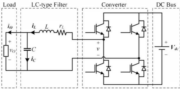
Fig. 1. Power stage of UPS inverter
