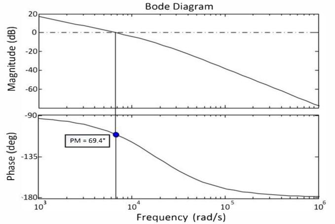
Fig. 6. Open-loop bode plot of the system
