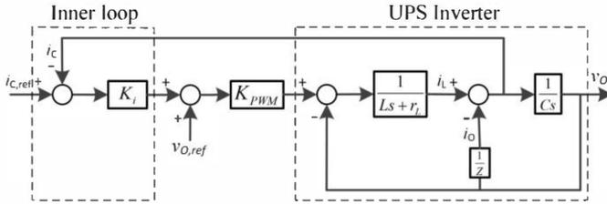
Fig. 4. Block diagram of UPS inverter with internal current loop
