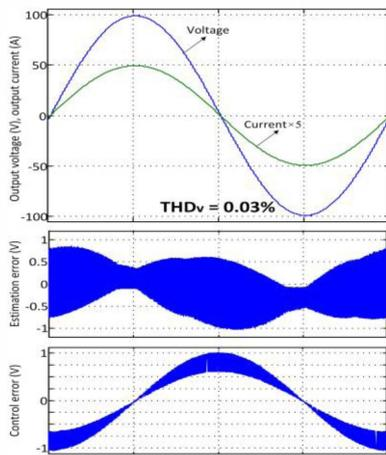
Fig. 8. Measured output voltage, current and errors under the nominal linear load
