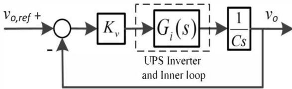
Fig. 5. Simplified block diagram of the proposed control system
