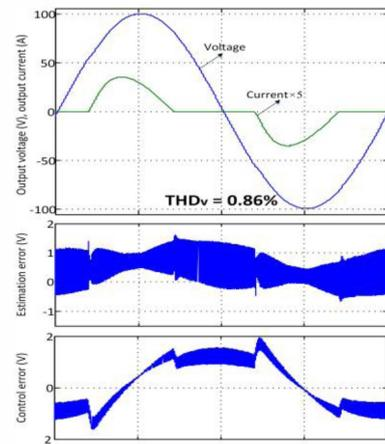
Fig. 10. Measured output voltage, current and errors under a highly non-linear load
