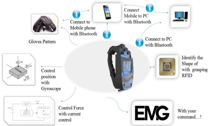
Fig.8. Connections of hand prosthesis
