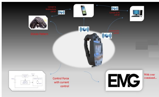
Fig.5. Connections of hand prosthesis
