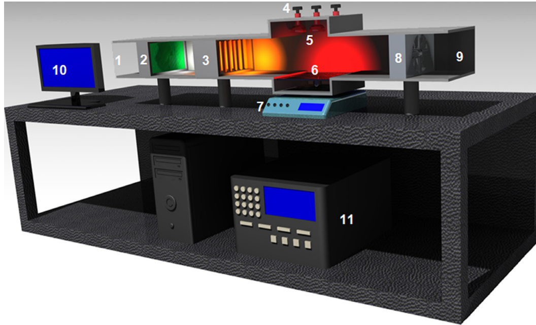
Fig. 1 – Experimental setup. (1 – fresh air inlet, 2 – air filter, 3 – heater, 4 – adjustment screws, 5 – infrared lamps, 6 – sample tray, 7 – digital balance, 8 – fan, 9 – air outlet, 10 – desktop computer, 11 – control unit).
