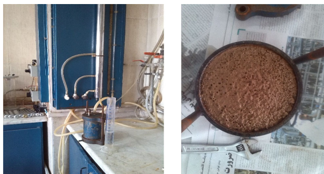
Fig. 6 The cell used for soil leaching (left) and sample G2 after leaching (right)
