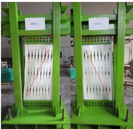
Fig. 10 Change in distortion direction due to the change in loading direction in the slit wall SSW-2
