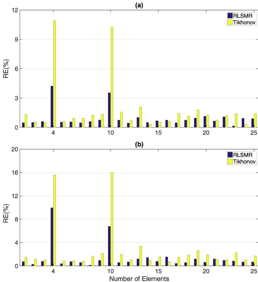
Fig. 9. The relative errors in damage quantities for the damage case 1: (a) 1% noisy data, (b) 5% noisy data.
