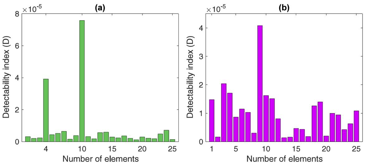
**Fig. 4.** The detectability of damage in the case 1: (a) the improved sensitivity of MSE, (b) the initial sensitivity of MSE.
