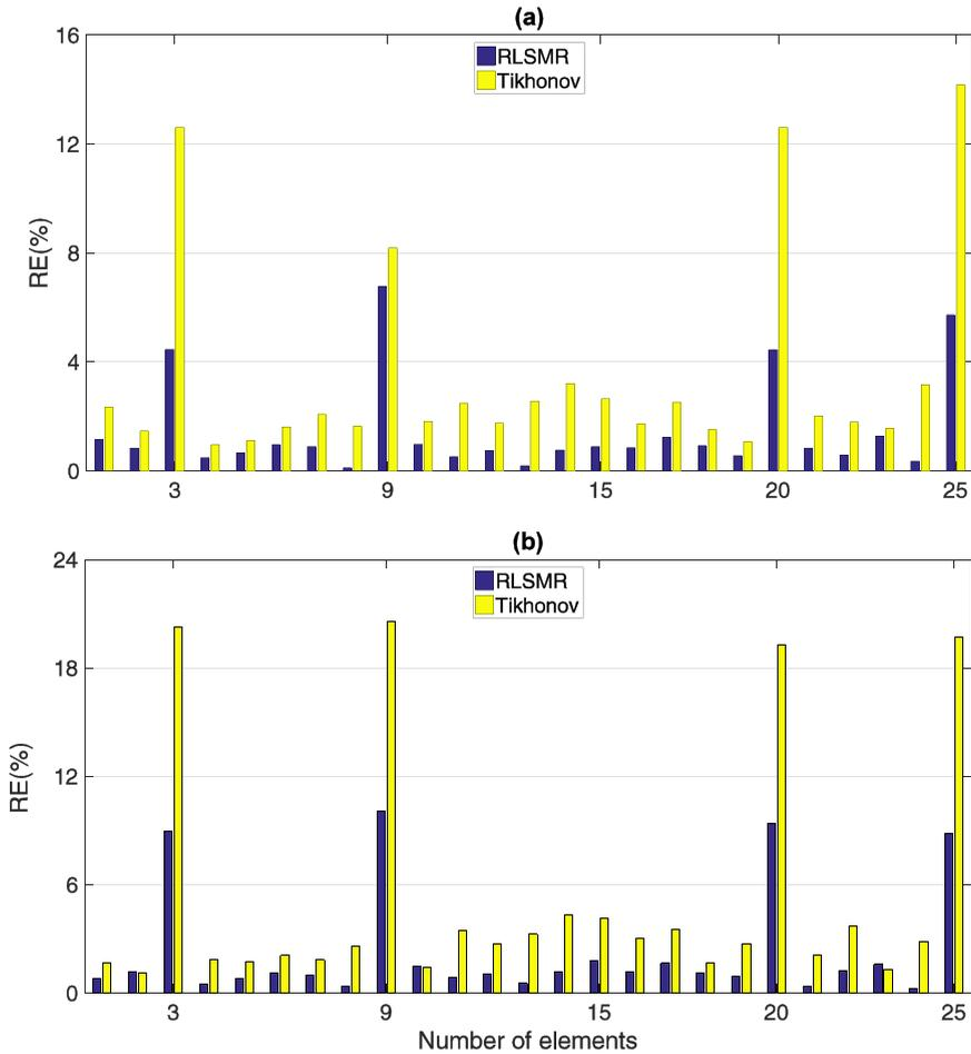
Fig. 10. The relative errors in damage quantities for the damage case 2: (a) 1% noisy data, (b) 5% noisy data.
