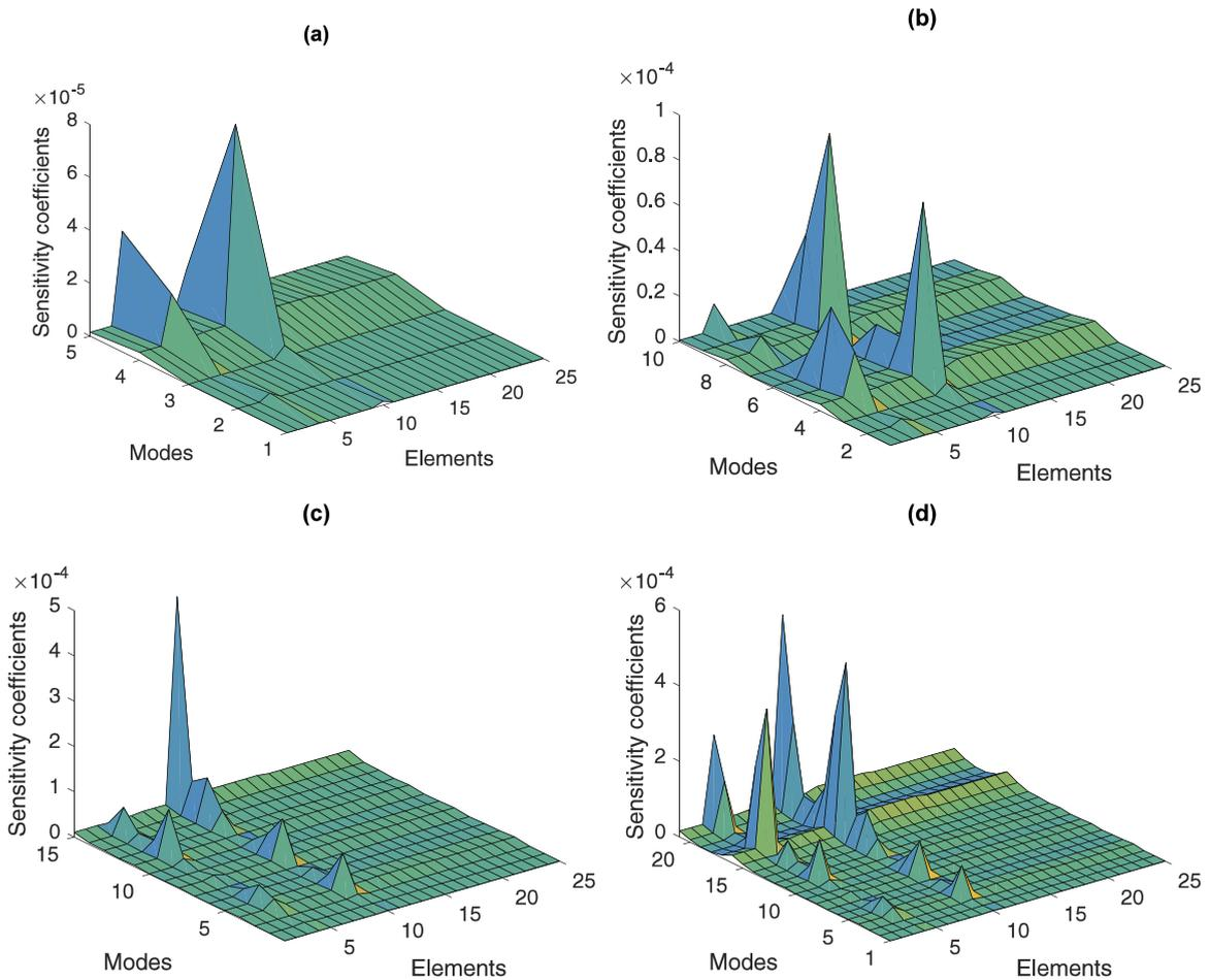
**Fig. 2.** The effect of measured modes on the improved sensitivity matrix of MSE in the damage case 1: (a) the first five modes, (b) the first ten modes, (c) the first fifteen modes, (d) the complete modes.
