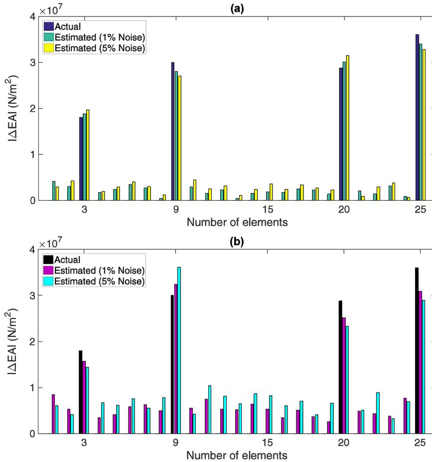
**Fig. 8.** Damage localization and quantification by the incomplete noisy modal parameters in the damage case 2: (a) RLSMR method, (b) Tikhonov regularization method.
