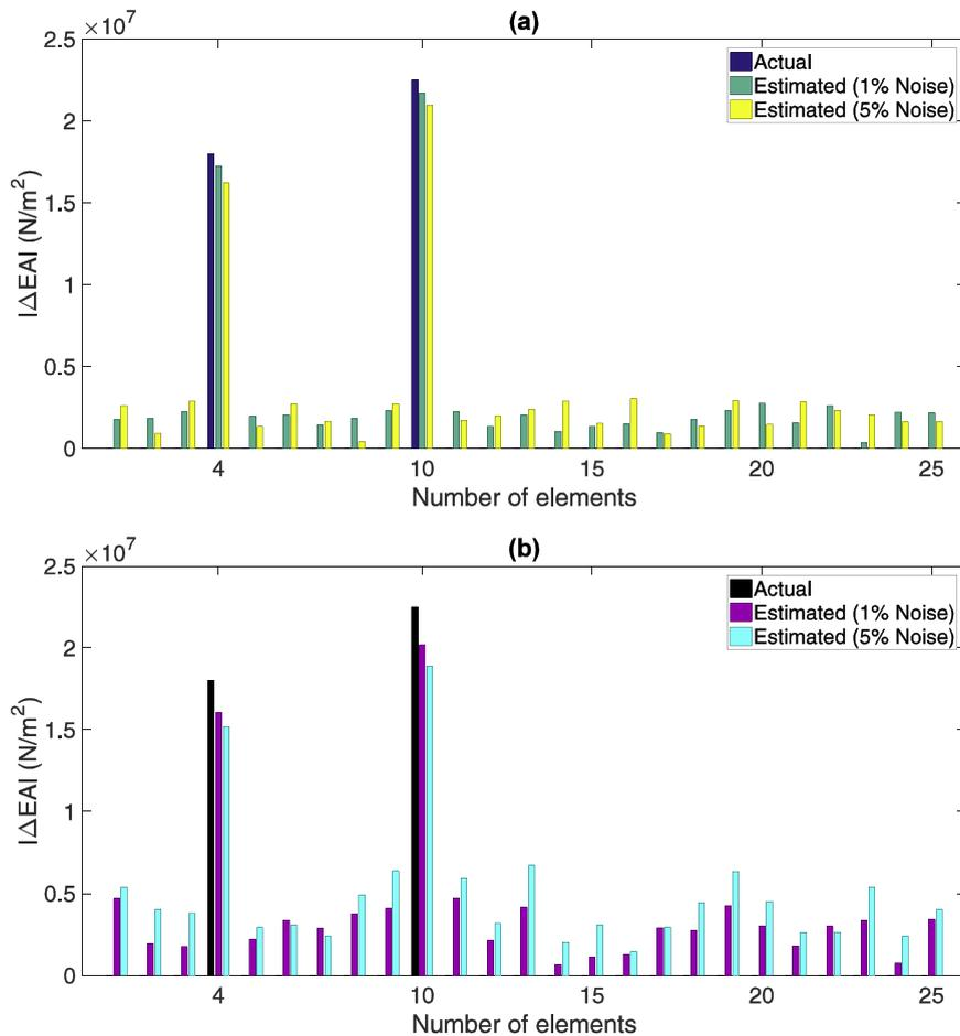
**Fig. 7.** Damage localization and quantification by the incomplete noisy modal parameters in the damage case 1: (a) RLSMR method, (b) Tikhonov regularization method.
