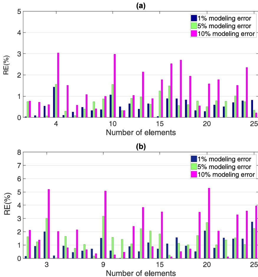
Fig. 12. The relative errors in damage quantities by considering the mass modeling errors: (a) case 1, (b) case 2.
