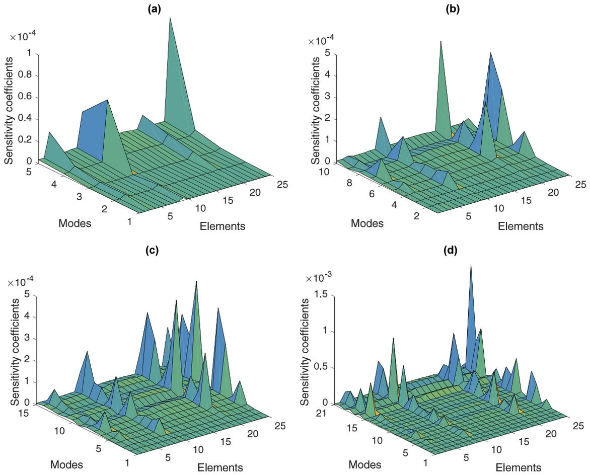
**Fig. 3.** The effect of measured modes on the improved sensitivity of matrix MSE in the damage case 2: (a) the first five modes, (b) the first ten modes, (c) the first fifteen modes, (d) the complete modes.
