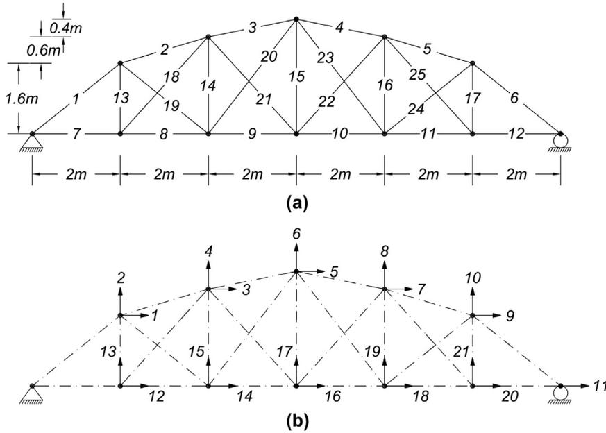
Fig. 1. The FE model of planner truss: (a) the model dimensions and elements, (b) the model DOFs.
