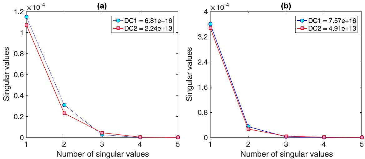
Fig. 6. The evaluation of ill-posed problem for the damage equation in: (a) 1% noise level, (b) 5% noise level (DC: Damage Case).
