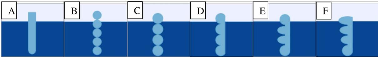
Fig. 1 : Six proposed geometries for OWSC. A to F represent Design A to Design F respectively. In all designs inertia is  $0.9\text{Kg.m}^2$
