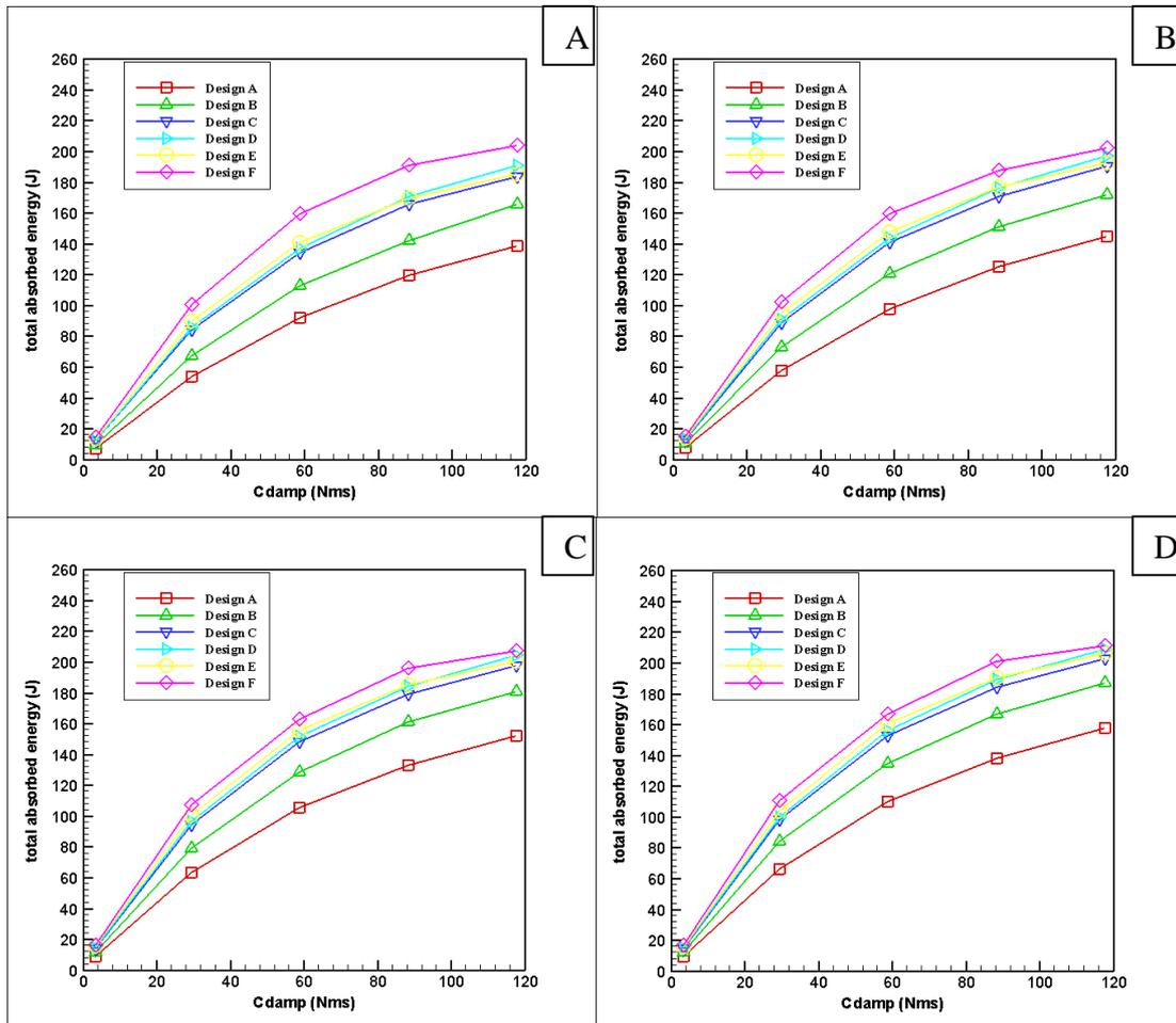
Fig. 2 : Total absorbed energy in 6s operation of wave maker that starts from still water for a 1m width OWSC in 6 different designs shown in fig. 1 versus damping coefficient. A:  $K=10.5\text{Nm/rad}$  , B:  $K=105\text{Nm/rad}$  , C:  $K=210\text{Nm/rad}$  , D:  $K=280\text{Nm/rad}$
