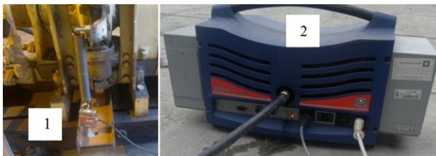
Fig. 1 The instrumentations for parameters measurements: 1- Load cell and 2- Diesel emission tester.
