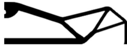
Fig. 5: MBB beam Stress-based design [7]
