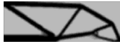
Fig. 4: MBB beam topological design \bar{\sigma}_1=350 MPa [3]
