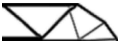
Fig. 2: Topological design by the proposed approach for \bar{\sigma}_1=350 MPa
