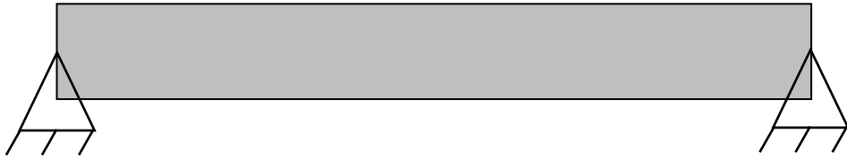
Fig. 2. Beam with simply supported ends
