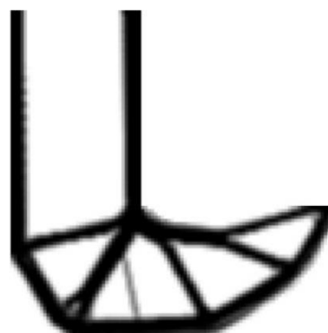
Fig. 9 Optimum layout of L-shaped beam with the presented method
