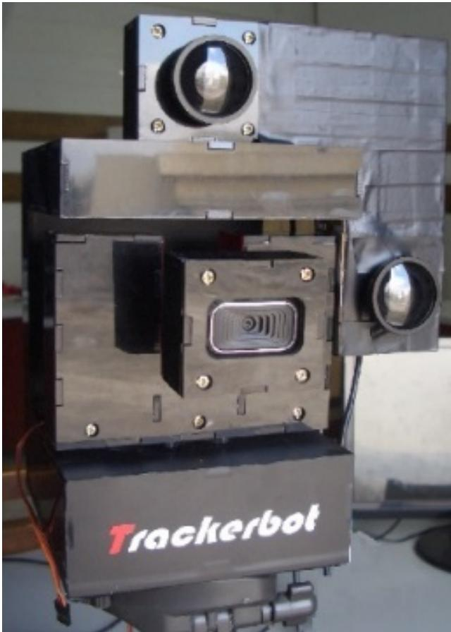
Fig. 2. The proposed camera system consist of two wide cameras and a central PTZ unit.
