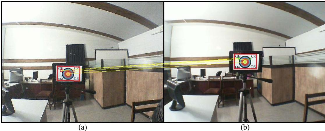
Fig. 9. A predefined target is located in the main wide camera (b). Afterwards, the target is registered in the second wide camera using the matched SURF feature and geometric transformation estimation (a).
