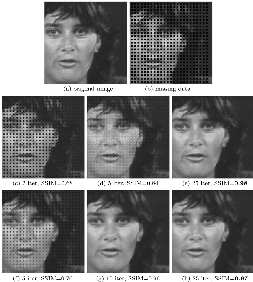
Fig. 10 Comparison of iterative thresholding (IT) algorithm as used in the ShearLab package and proposed method. Both methods use the same shearlet system with 4 scales. Image (a) shows the original test image and (b) displays the image distorted image. Second row shows intermediate results of the proposed algorithm combining iterative thresholding and TGV. Last row shows intermediate results of different iterations of the IT algorithm
