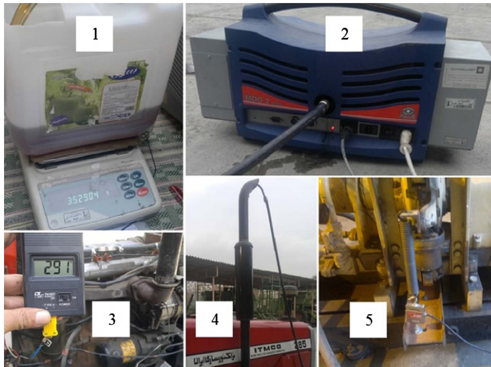
Fig. 2. The instrumentations for the parameters measurements: 1 – Digital scale to measure fuel consumption, 2 – Diesel emission tester, 3 – Temperature monitor and sensor, 4 – Emission probe and 5 – Load cell.
