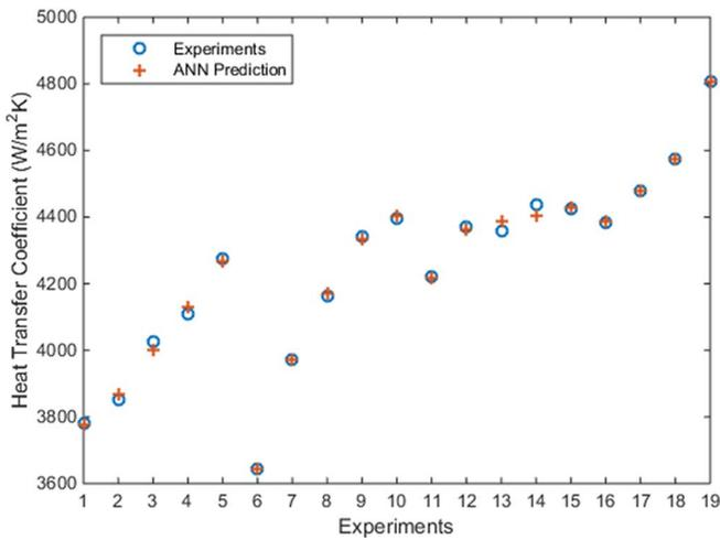
Fig. 7. The experimental results versus the network outputs for the train data set to predict the heat transfer coefficients.
