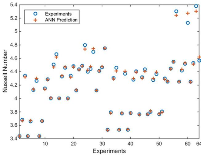
Fig. 12. The experimental results versus the network outputs for the train data set to predict the Nusselt number.
