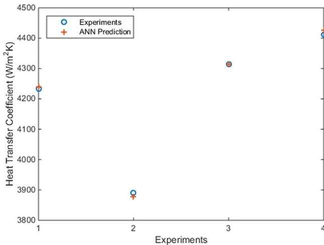
Fig. 8. The experimental results versus the network outputs for the test data set to predict the heat transfer coefficients.
