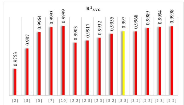
Fig. 9. Average of the correlation coefficients for the train data sets after 10 runs of each network structure to predict the Nusselt number.
