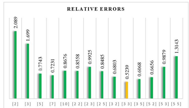
Fig. 11. Average of the relative errors for the test data sets after 10 runs of each network structure to predict the Nusselt number.
