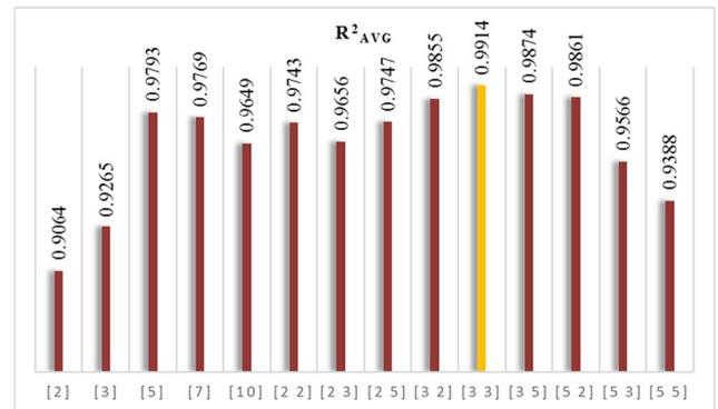
Fig. 10. Average of the correlation coefficients for the test data sets after 10 runs of each network structure to predict the Nusselt number.
