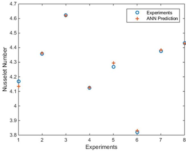
Fig. 13. The experimental results versus the network outputs for the test data set to predict the Nusselt number.
