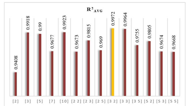
Fig. 5. Average of the correlation coefficients for the test data sets after 10 runs of each network structure to predict the heat transfer coefficients.
