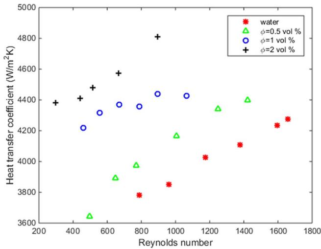
Fig. 2. Experimental heat transfer coefficient versus Reynolds number for heating rate of 69.1 W [30].
