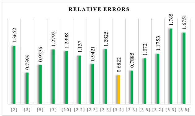
Fig. 6. Average of the relative errors for the test data sets after 10 runs of each network structure to predict the heat transfer coefficients.
