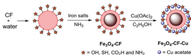
Scheme 1. Preparation of \text{Fe}_3\text{O}_4\text{-CF-Cu} MNPs.
