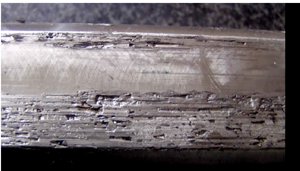
Fig. 6 Wear scratches on rails [30]
