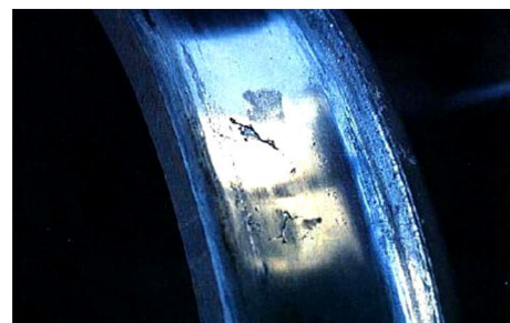
Fig. 10 Delamination wear of wheel [30]
