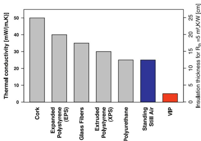
Fig. 3. Thermal efficiency of insulation materials: thermal conductivity and insulation width for a fixed thermal resistance of  $5 \text{ m}^2 \cdot \text{K/W}$  (Reprinted from Bouquerel et al. [14] with permission from the publisher).
