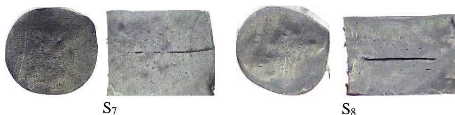
Figure 2. Observed damages of NBR vulcanized samples as O-ring and Ring-type specimens under the modified RGD test.
