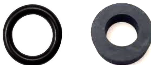
Figure 1. Two specimen geometry as O-ring and Ring-type of rubber samples used in modified RGD test
