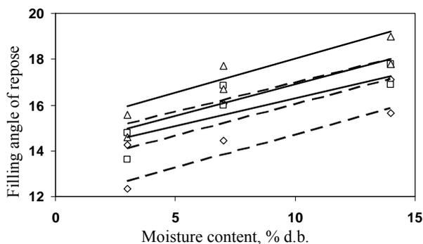
Fig. 22 The filling angle of repose of Azar gol sunflower seed and its kernel as a function of moisture content and size ( $\diamond$ , large;  $\square$ , medium;  $\triangle$ , small; —, seed; ---, kernel.).
