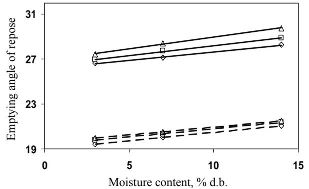
Fig. 18 The emptying angle of repose of Fandoghi sunflower seed and its kernel as a function of moisture content and size (◇, large; □, medium; △, small; —, seed; - - -, kernel.).
