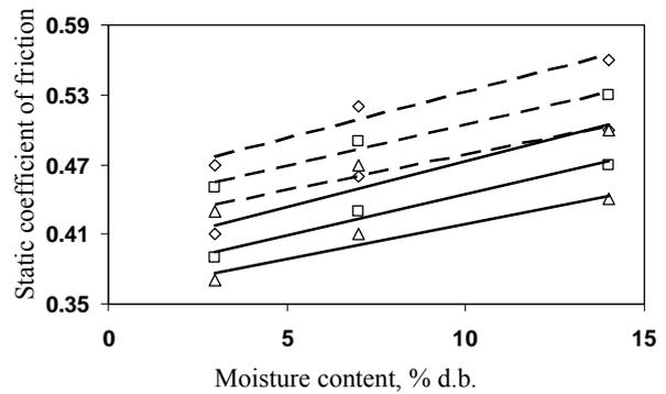
Fig. 13 The static coefficient of friction of Azar gol sunflower seed and its kernel on polyethylene surface as a function of moisture content and size (◇, large; □, medium; △, small; —, seed; ---, kernel.).
