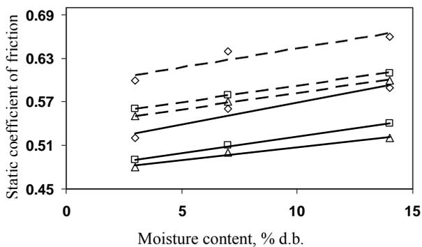
Fig. 15 The static coefficient of friction of Fandoghi sunflower seed and its kernel on rubber surface as a function of moisture content and size (◇, large; □, medium; △, small; —, seed; - - -, kernel).
