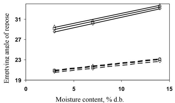
Fig. 20 The emptying angle of repose of Shahroodi sunflower seed and its kernel as a function of moisture content and size (◇, large; □, medium; △, small; —, seed; - - -, kernel.).
