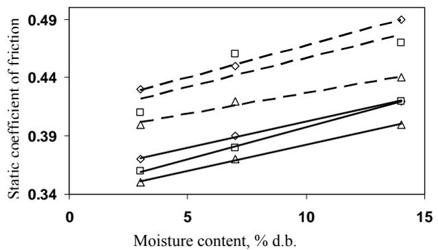
Fig. 11 The static coefficient of friction of Shahroodi sunflower seed and its kernel on galvanized iron sheet as a function of moisture content and size (◇, large; □, medium; △, small; —, seed; ---, kernel.).
