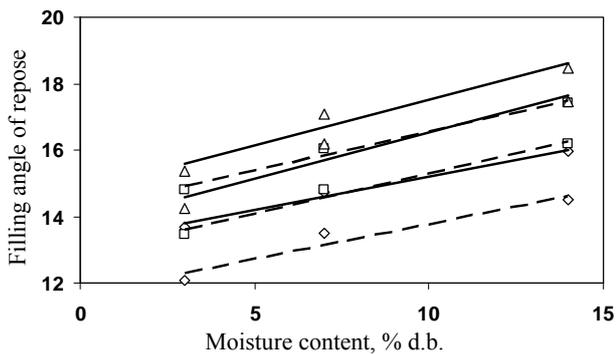
Fig. 21 The filling angle of repose of Fandoghi sunflower seed and its kernel as a function of moisture content and size ( $\diamond$ , large;  $\square$ , medium;  $\triangle$ , small; —, seed; ---, kernel.).
