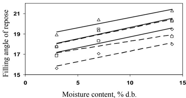
Fig. 23 The filling angle of repose of Shahroodi sunflower seed and its kernel as a function of moisture content and size ( $\diamond$ , large;  $\square$ , medium;  $\triangle$ , small; —, seed; ---, kernel.).
