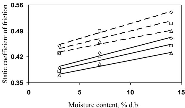
Fig. 12 The static coefficient of friction of Fandoghi sunflower seed and its kernel on polyethylene surface as a function of moisture content and size (◇, large; □, medium; △, small; —, seed; ---, kernel.).
