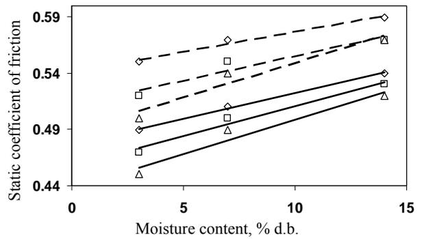
Fig. 17 The static coefficient of friction of Shahroodi sunflower seed and its kernel on rubber surface as a function of moisture content and size (◇, large; □, medium; △, small; —, seed; - - -, kernel).
