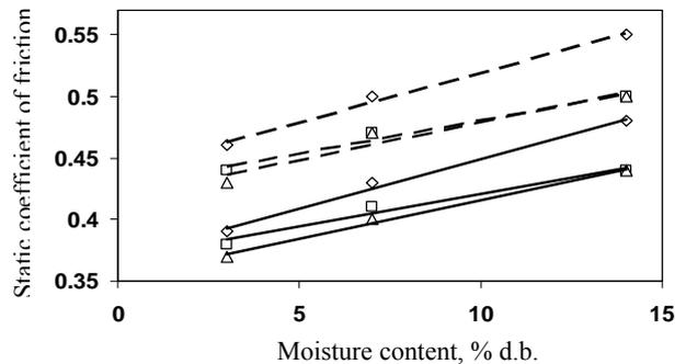
Fig. 14 The static coefficient of friction of Shahroodi sunflower seed and its kernel on polyethylene surface as a function of moisture content and size (◇, large; □, medium; △, small; —, seed; ---, kernel.).
