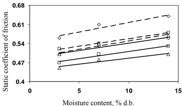
Fig. 16 The static coefficient of friction of Azar gol sunflower seed and its kernel on rubber surface as a function of moisture content and size (◇, large; □, medium; △, small; —, seed; - - -, kernel).
