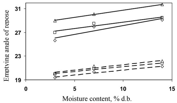
Fig. 19 The emptying angle of repose of Azar gol sunflower seed and its kernel as a function of moisture content and size (◇, large; □, medium; △, small; —, seed; - - -, kernel.).
