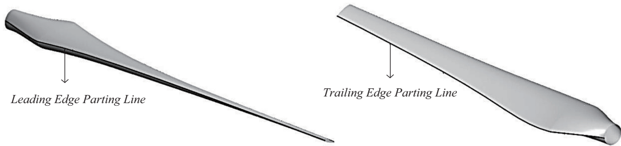
Fig. 2 Parting Lines in the leading and trailing edges of a typical wind turbine blade.
