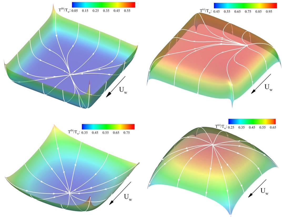
**Figure 4.** Ballistic heat flow lines overlaid on the ballistic temperature field (left) and collision heat flow lines overlaid on the collision temperature field (right) for  $\text{Kn} = 0.05$  (up) and  $\text{Kn} = 0.5$  (down).
