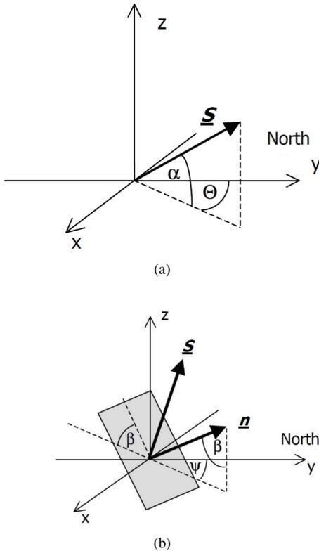
Fig. 1. Sun position unit vector and panel's normal vector [18]: (a)  $\underline{S}$  is the unit vector pointing the sun. The sun's azimuth and altitude angles are shown, (b)  $\underline{n}$  is the normal vector of the module. The panel's tilt and orientation angles are shown.
