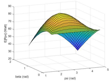
Fig. 6. The expected value of produced power in the feasible range calculated by Monte Carlo method.
