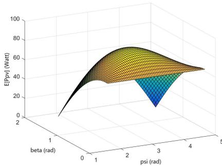
Fig. 4. The expected value of produced power in the feasible range calculated by SPC method.
