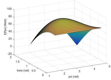
Fig. 5. The expected value of produced power in the feasible range calculated by CVE method.
